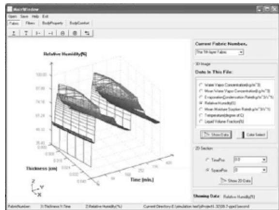
Figure 14. Relative humidity distribution at the first layer of garment in PPC1
