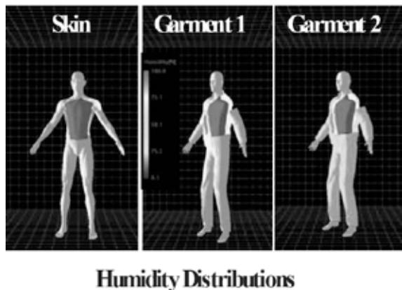
Figure 16. Humidity distributions at the skin surface, the first garment surface and the second garment surface of in PPC1 visualized on the 3D human manikin
