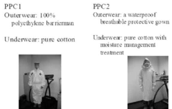
Figure 4. Computational thermal ergonomic design of personal protective clothing
