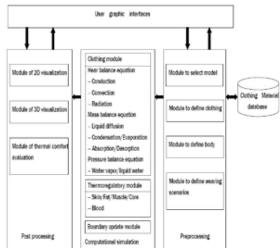
Figure 3. Software architecture in the textile thermal bioengineering CAD system
