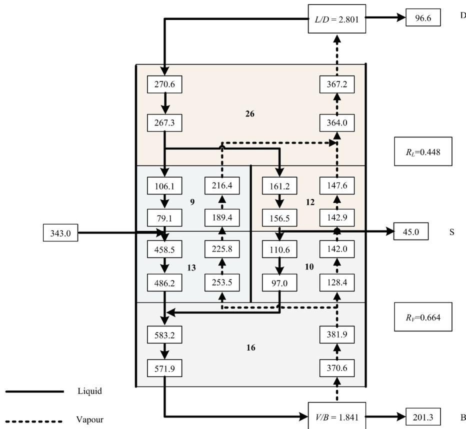
Fig. 12 – Internal configuration with material balance of a DWC, indicating liquid and vapour flow rates at the top and bottom, and the number of stages of each section as well as resulting liquid and vapour splits
