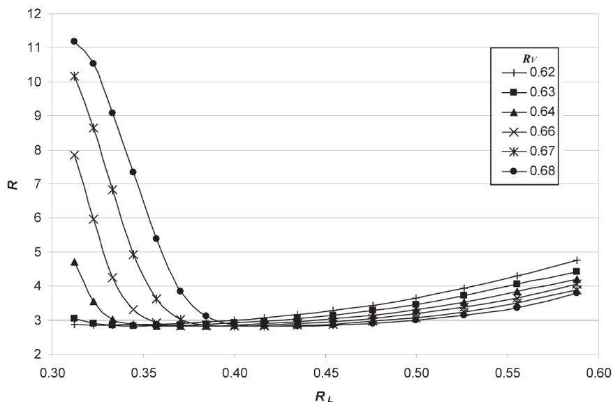
Fig. 9 – Operating reflux as a function of the liquid split with vapour split as a parameter
