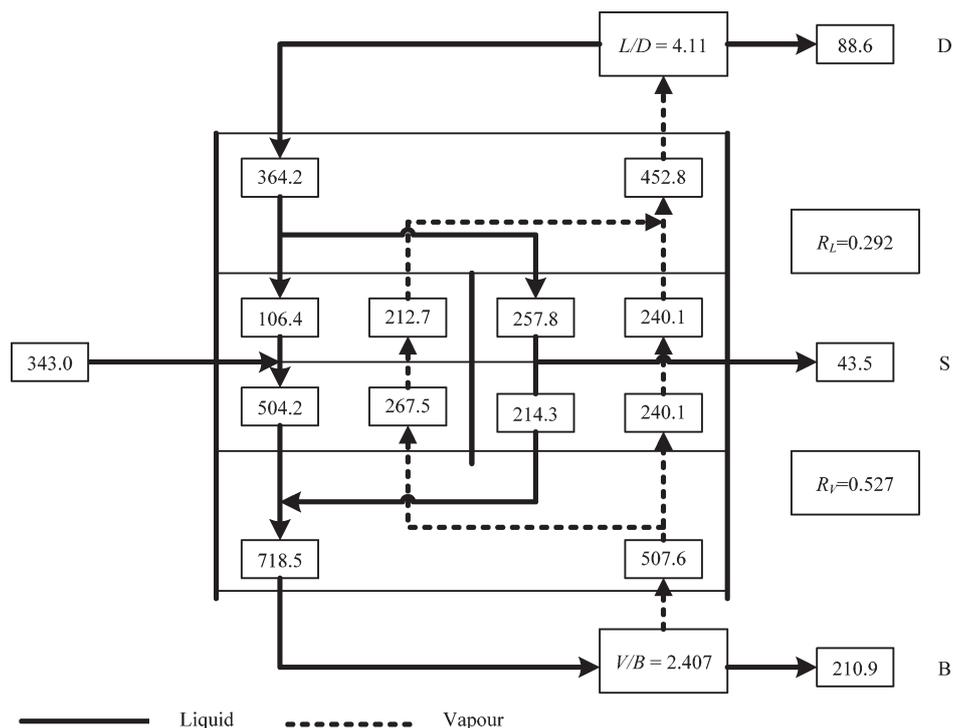
Fig. 6 – Internal values of molar flow rates and phase splits according to  $V_{min}$  diagram, initial values for rigorous simulation
