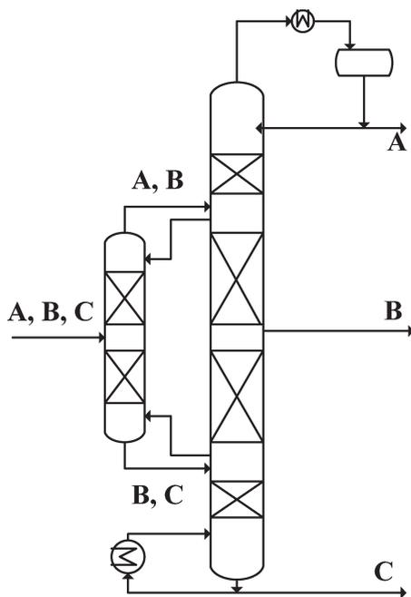
Fig. 2 – Petlyuk arrangement with thermally coupled prefractionator and main column
