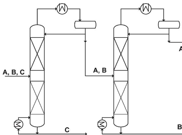
Fig. 1 – Conventional three-component separation arrangement
