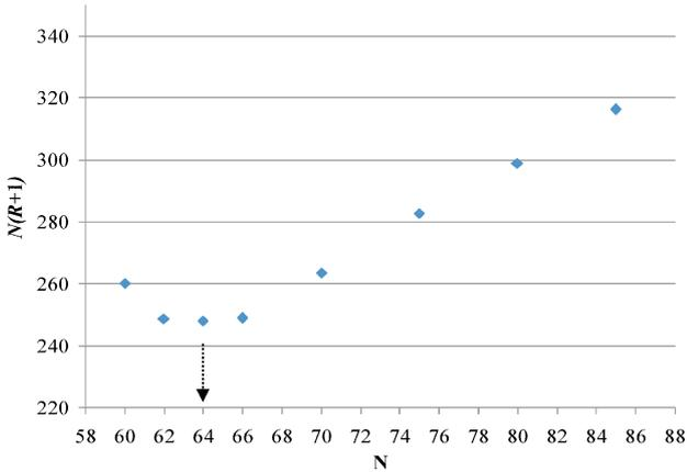
Fig. 11 – Determination of the optimum number of equilibrium stages for a DWC
