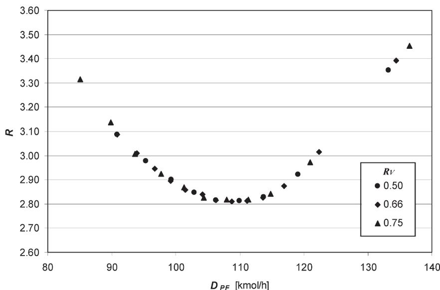
Fig. 10 – Operating reflux as a function of net flow rate in the prefractionator for various vapour split values
