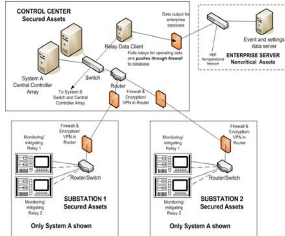
Figure 10. Secure communications architecture
