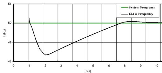
Figure 7. System and sub-system frequency response, an islanding scenario with consumption surplus
