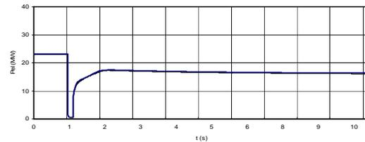
Figure 8. Electrical power production response of units G3 and G4, an islanding scenario with generation surplus
