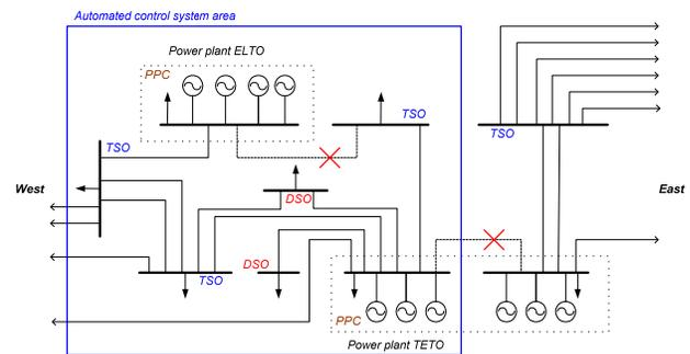
Figure 1. Central Zagreb 110 kV transmission system
