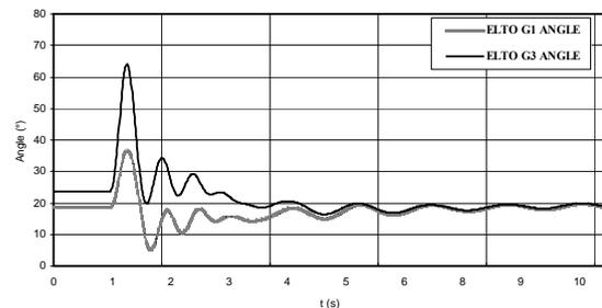
Figure 5. Angle response of units G1 and G3, three-phase short-circuit fault on 110 kV busbars in SS Jarun,  $T_{cr} = 160$  ms
