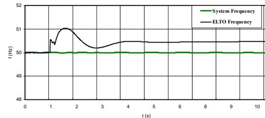
Figure 9. System and sub-system frequency response, an islanding scenario with generation surplus
