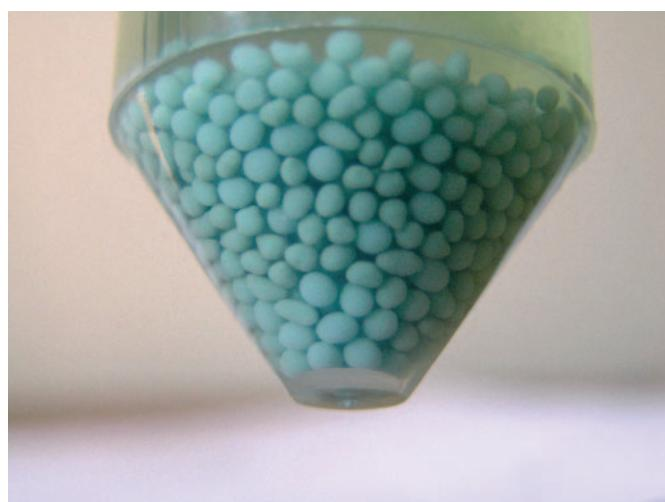
**Figure 2.** Mixed copper-loaded alginate/chitosan capsules
