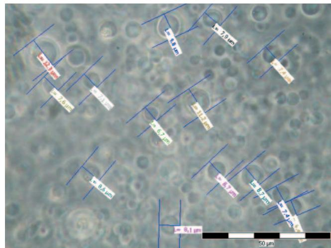
**Figure 1.** Size determination of copper-loaded chitosan based microcapsules
