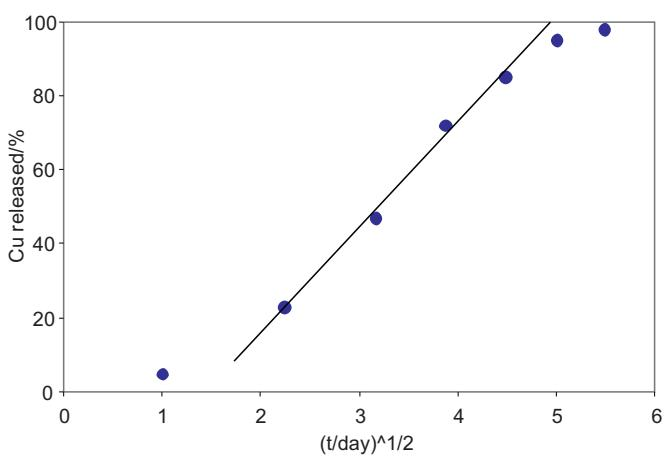
Figure 5. Higuchi diagram of copper release from alginate/chitosan capsules
