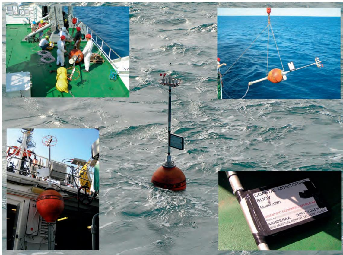
Figure 5. Coastal meteorological buoy, the way it is secured on the deck (bottom left) attached to the crane (top left), lowered into the sea (top right) and floats (background).
