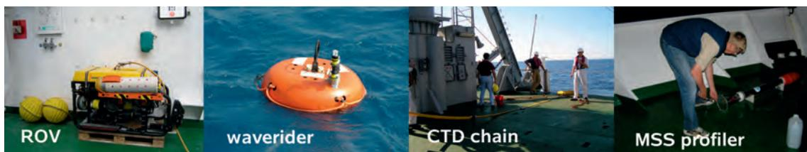
Figure 8. From left to right: ROV, waverider, lowering of the CTD chain and microstructure measuring system.
