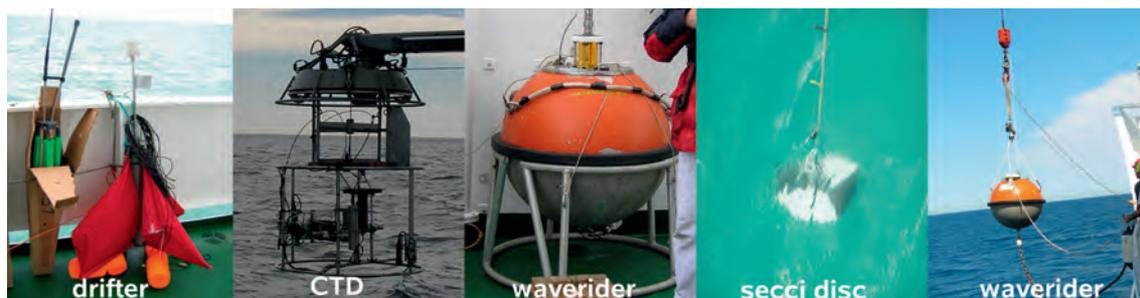
Figure 7. From left to right: lagrangian drifters, CTD, waverider on deck, Secci disc, waverider lowered to the sea.
