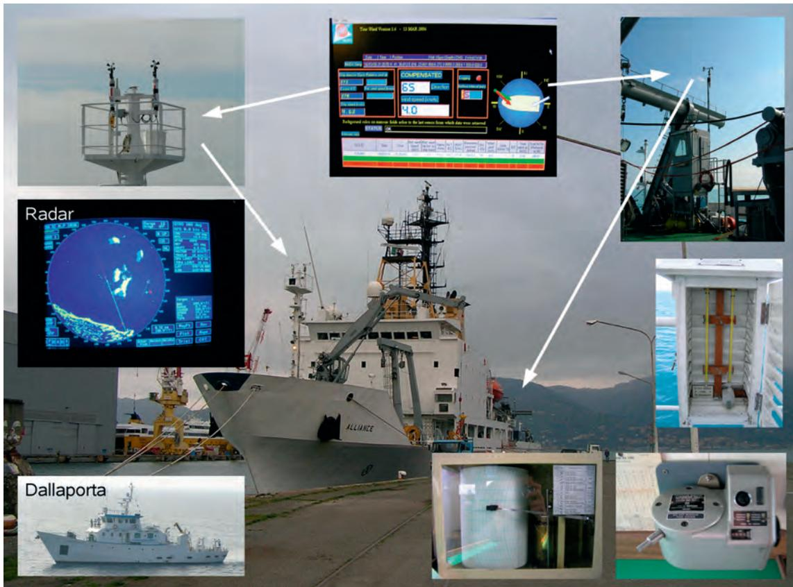
Figure 4. NRV Alliance and attached meteorological instruments, display from automatic meteorological station, ship's radar display and Dallaporta research vessel.
