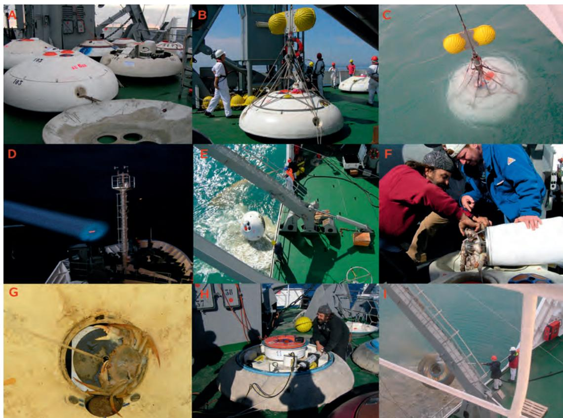
Figure 6. Process of assembling the SEPTR on board (A), attaching it to the crane (B), lowering it to the sea bottom (C), the search for it (D) and retrieval (E) with some examples how marine life can endanger the instruments operations (F) and (G) causing malfunction of the instrument. Assembling (H) and retrieval (I) of Barny are also shown.
