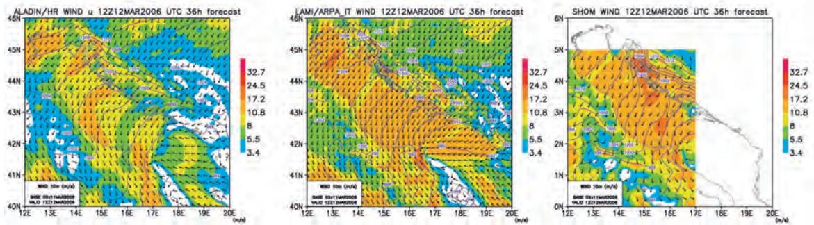
Figure 13. Forecast 10 m wind for 12 UTC on 12<sup>th</sup> March 2006 using Aladin-Croatia (left), LAMI (centre) and Aladin-France (right).
