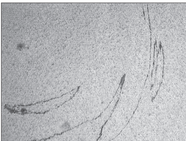
Figure 18 Microstructure of specimen No. 9, resulted after the influence of the pin
