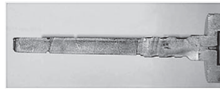
Figure 6 Heat treated planetary shaft - longitudinal cross-section
