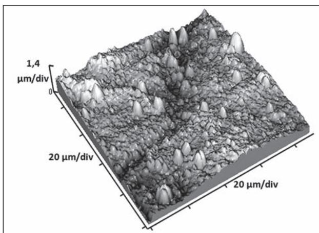
Figure 1 AFM image of a TiN coating implanted with nitrogen
