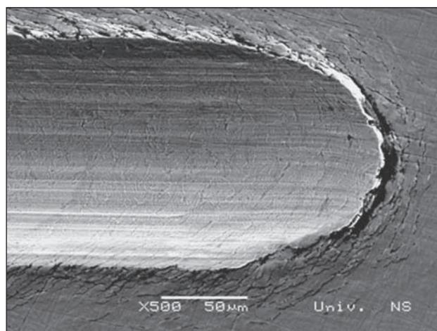
Figure 3 Delamination of coating
