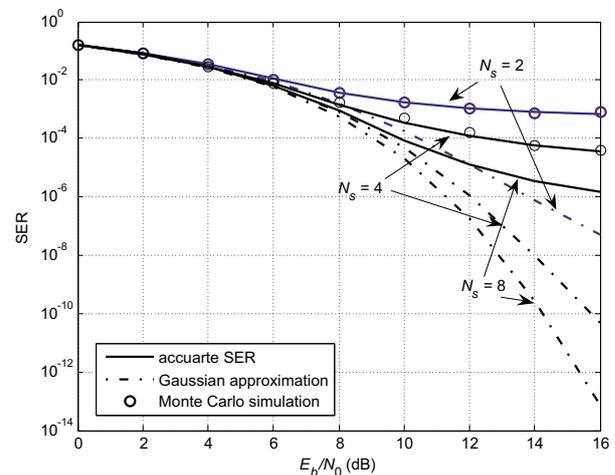
**Figure 2** Accurate analytical SER of PPAM versus  $E_b/N_0$  with system parameters  $N = M = 2$ ,  $N_s = 2, 4, 8$ ,  $T_f = 50$  ns,  $T_c = N \cdot 0,9$  ns,  $N_h = 8$ ,  $\tau_p = 0,2877$  ns,  $\delta = 0,72$  ns,  $N_u = 8$
