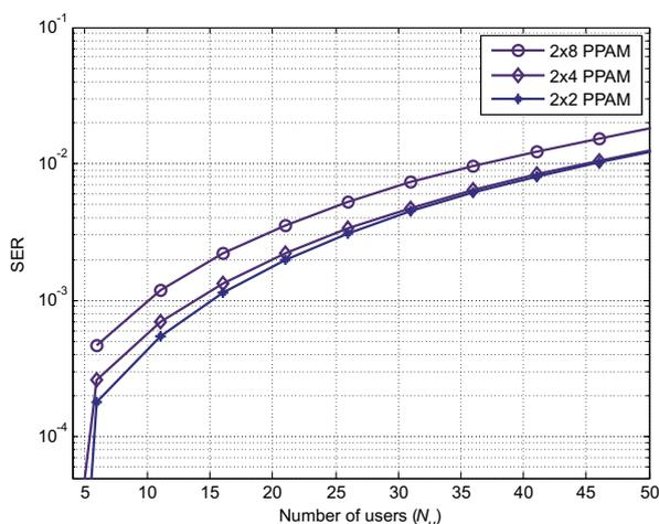
**Figure 4** Comparison of PPAM with different modulation level versus  $N_u$  for fixed bit rate (15 Mb/s). System parameters are  $N_s = 2$ ,  $T_c = N \cdot 0,9$  ns,  $\tau_p = 0,2877$  ns,  $\delta = 0,72$  ns, SNR = 15 dB
