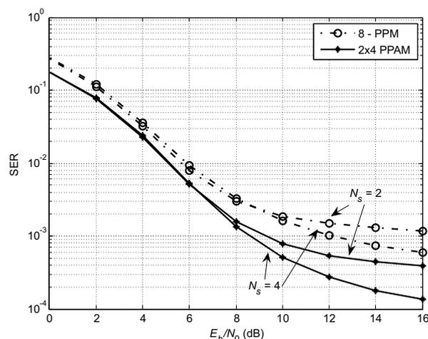
**Figure 5** Comparison of PPAM and orthogonal PPM with different modulation level versus  $E_b/N_0$  for fixed bit rate (15 Mb/s). System parameters are,  $T_c = N \cdot 0,9$  ns,  $\tau_p = 0,2877$  ns,  $\delta = 0,72$  ns,  $N_u = 8$ , for  $N_s = 2$ ,  $N_h = 13$  (6 for PPM) and for  $N_s = 4$ ,  $N_h = 6$  (3 for PPM)
