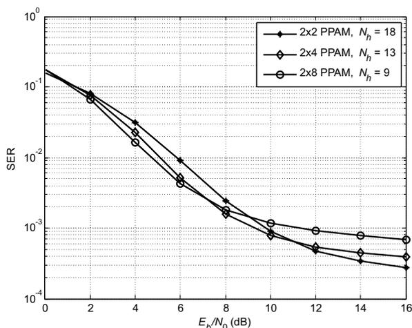
**Figure 3** Comparison of PPAM with different modulation level versus  $E_b/N_0$  for fixed bit rate (15 Mb/s). System parameters are  $N_s = 2$ ,  $T_c = N \cdot 0,9$  ns,  $\tau_p = 0,2877$  ns,  $\delta = 0,72$  ns,  $N_u = 8$
