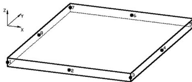
Figure 6 Schematic representation of the used "shell" element
