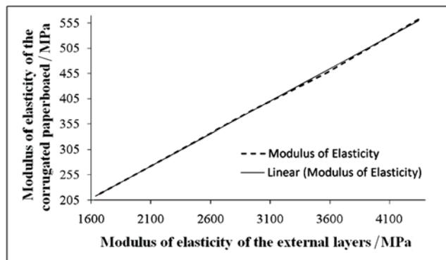
Figure 13 Effect of "liners" on the modulus of elasticity
