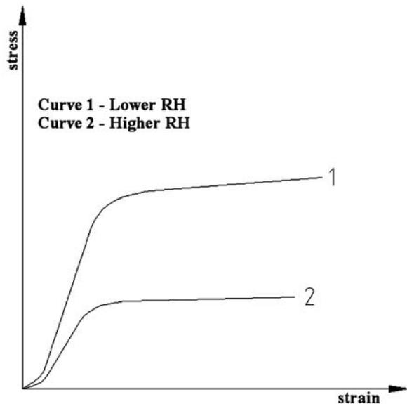
Figure 3 "Stress-strain" curves of paper at different levels of moisture
