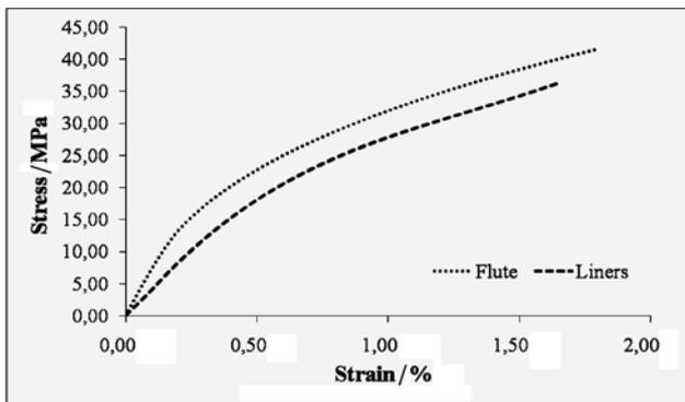
Figure 9 "Stress – strain" curves used for different layers [3]
