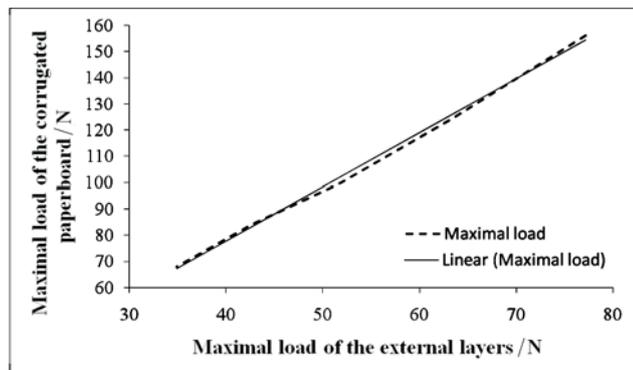
Figure 14 Changing of the maximal load of the liners and the corrugated paperboard panel
