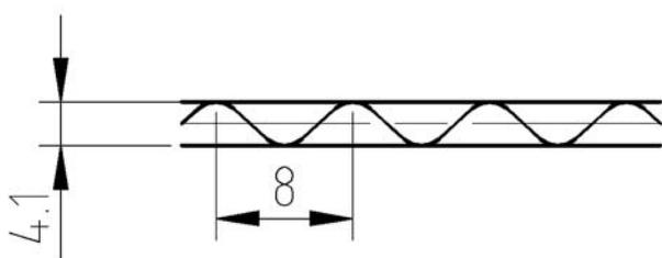
Figure 4 Geometrical parameters of "C" flute type used for the modeling – dimensions are in millimeters
