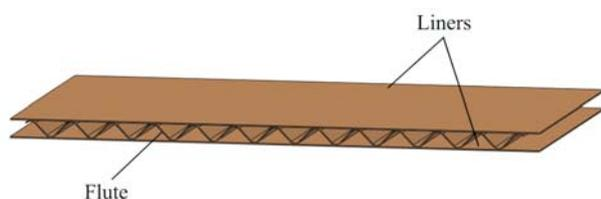
Figure 1 Structure of the corrugated paperboard
