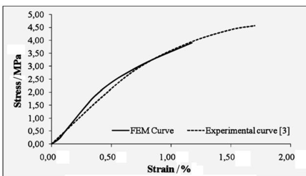
Figure 10 Comparison between the experimental and FEM complex curves for the corrugated paperboard
