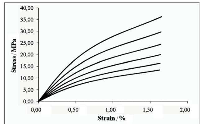
Figure 11 Used "stress – strain" curves for the liners
