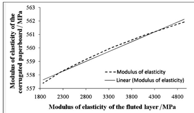
Figure 17 Effect of the internal layer on the modulus of elasticity
