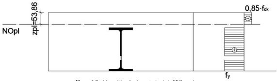
Figure 6 Position of the plastic neutral axis in SPC specimen Slika 6. Položaj plastične neutralne osi u SPC uzorku
