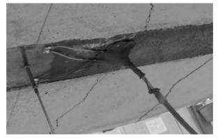
Figure 14 Strain gauges fastened to lower flange Slika 14. Mjerne otporne trake pričvršćene za donju prirubnicu
