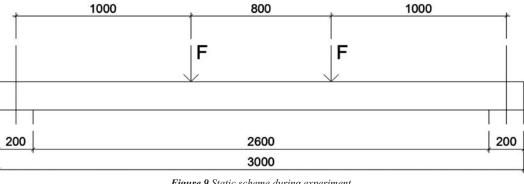
Figure 9 Static scheme during experiment Slika 9. Statička shema tijekom ekspererimenta
