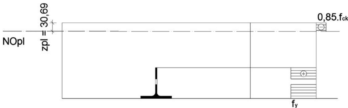
Figure 8 Position of the plastic neutral axis for SPP specimen
