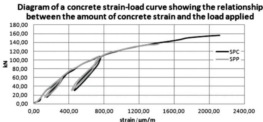
Figure 20 Diagram of a concrete strain-load curve showing the relationship between the amount of concrete strain and the load applied
