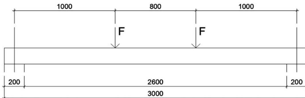
Figure 9 Static scheme during experiment
