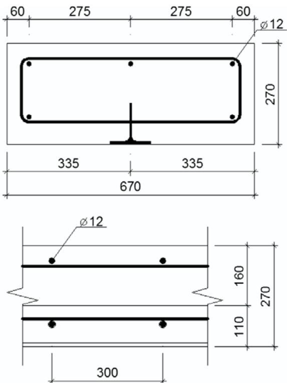
Figure 2 Cross section and longitudinal section of SPP specimen
