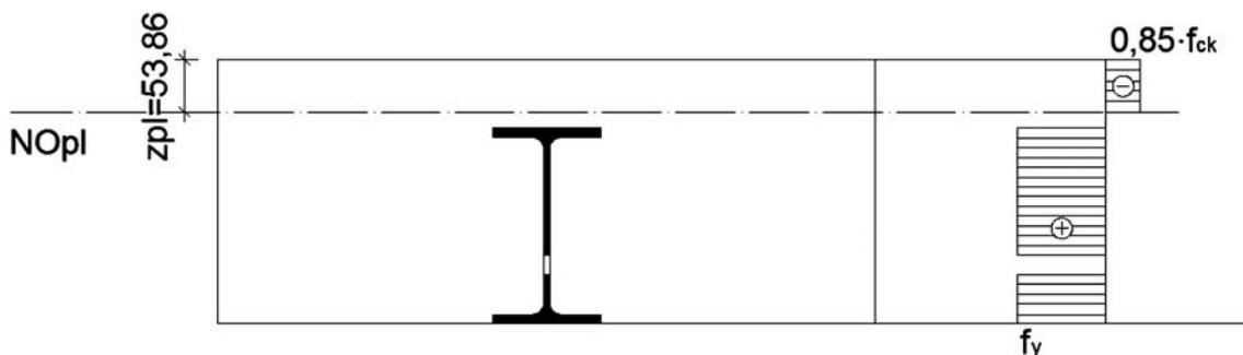
Figure 6 Position of the plastic neutral axis in SPC specimen
