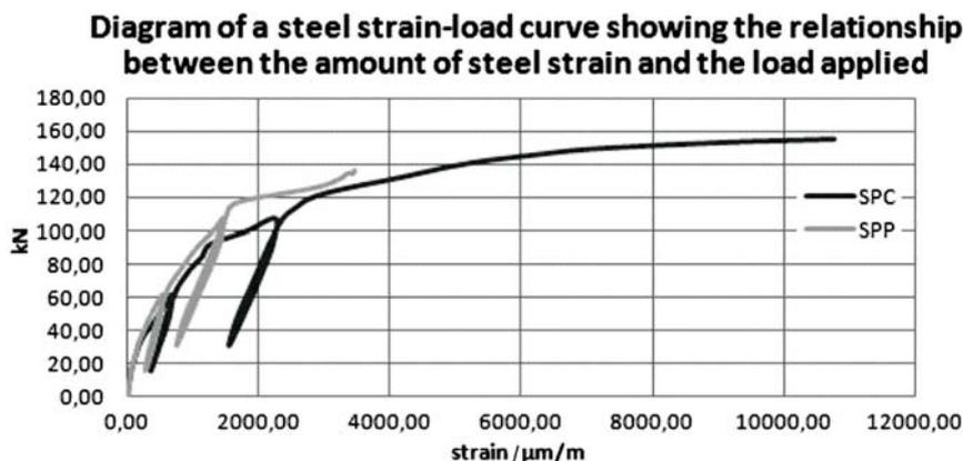
Figure 19 Diagram of a steel strain-load curve showing the relationship between the amount of steel strain and the load applied
