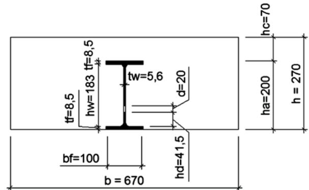
Figure 5 Cross section dimensions for SPC specimen
