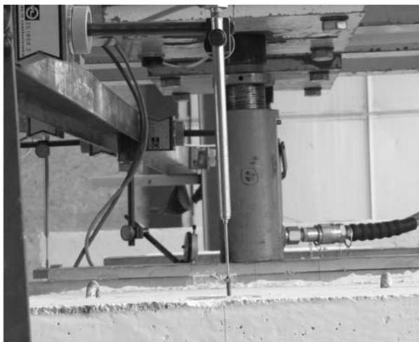
Figure 13 Inductive sensor above the support
