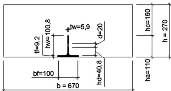
Figure 7 Cross section dimensions for SPP specimen
