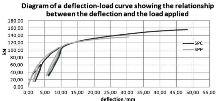
Figure 18 Diagram of a deflection-load curve showing the relationship between the deflection and the load applied
