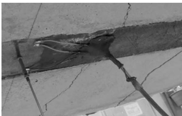
Figure 14 Strain gauges fastened to lower flange
