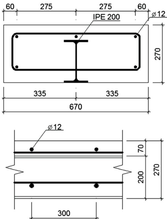
Figure 1 Cross section and longitudinal section of SPC specimen
