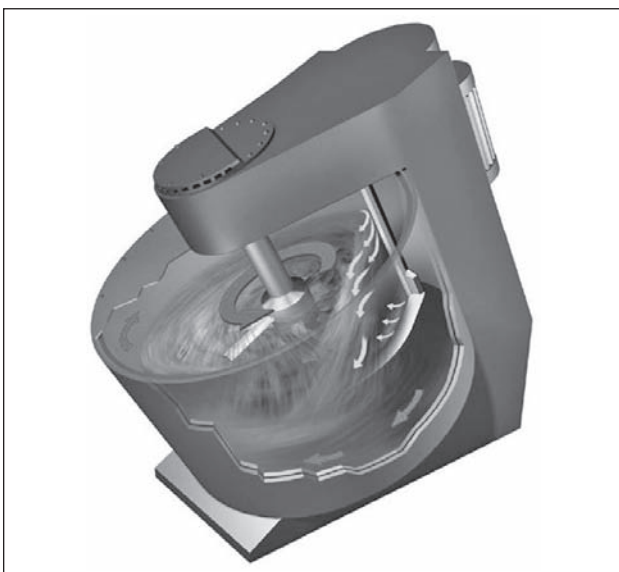
Figure 1 Principle of operation of the intensive mixer [13].
