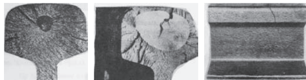
Figure 3 Progressive transverse cracking
