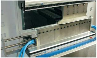
Figure 1 400 mm diode laser assisted bending tool
