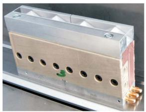
Figure 2 Diode laser inset with 100 mm length
