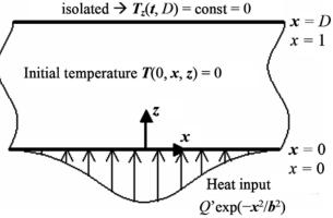
Figure 8 2-dimensional heat-conduction with Gaussian heat input on lower surface and isolated upper surface
