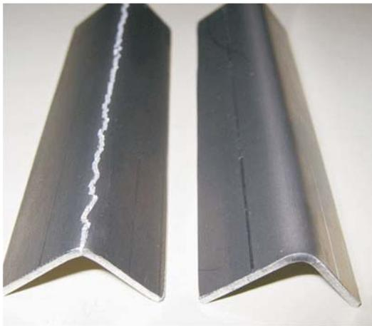
Figure 6 Comparison of cold (crack) and laser assisted bending of the Mg-alloy AZ31
