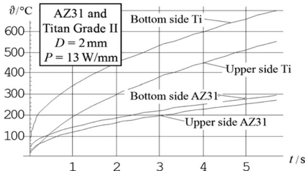
**Figure 9** Simulation of heating curves at the bottom and upper side for Mg- and Ti- sheet metals
