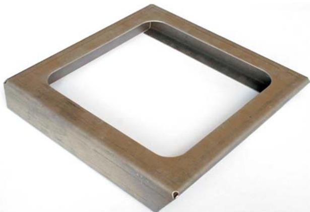
Figure 7 Bending part made of AZ31 with 6 bends with ~250 mm length
