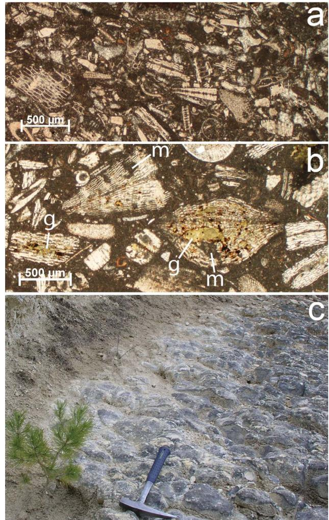
**Figure 21:** T2S. Condensation features. **a** – Thin-section showing fragmented skeletal remains (mainly foraminifera), inferred to have been produced by scavengers as a consequence of decreased sedimentation rates close to maximum transgression. **b** – Borings in foraminifera may contain mudstone (m) and/or glauconite (g). **a** and **b**: Section 2I in Figs. 6 and 16. **c** – Bioturbated hardground surface at the top of the transgressive unit (TST). Section 2B in Figs. 6 and 16.
