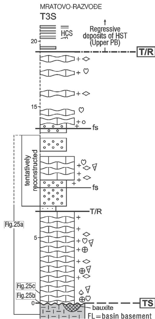
**Figure 24:** Log of T3S (Mratovo-Razvođe). Reconstructed using smaller, partial sections and isolated outcrops located along 5km long, discontinuous stretch of T3S (labelled “3” in Fig. 16). The basement is mostly represented by Middle Eocene Foraminiferal Limestones (FL) and locally, by Upper Cretaceous limestones. For other symbols see Fig. 16.
