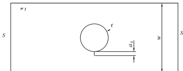
**Figure 2.** Geometry of cracked structural element
