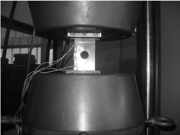
**Figure 4.** Experimental measuring of crack propagation with use of measuring foils
