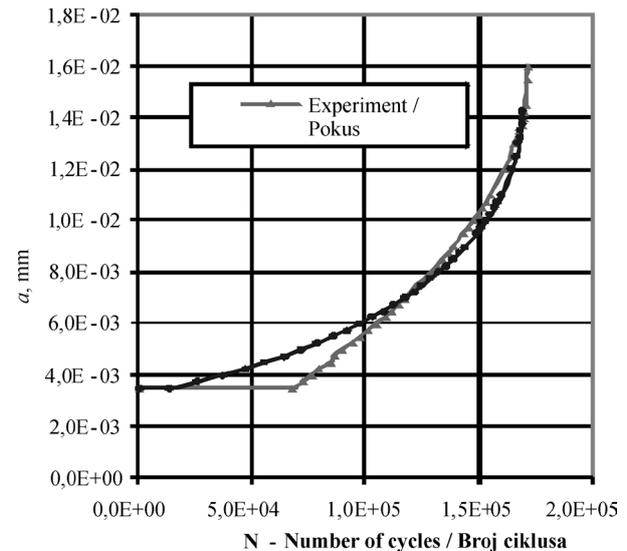
**Figure 6.** Analysis of crack propagation: Comparison of computation and experimental results ( $K_c = 139$ )
