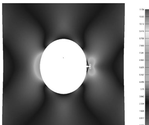
**Figure 3.** Stress distribution for structural element with a circular hole and one crack ( $F = 5\ 200$  N and  $a = 0.00127$  m) using finite element analysis
