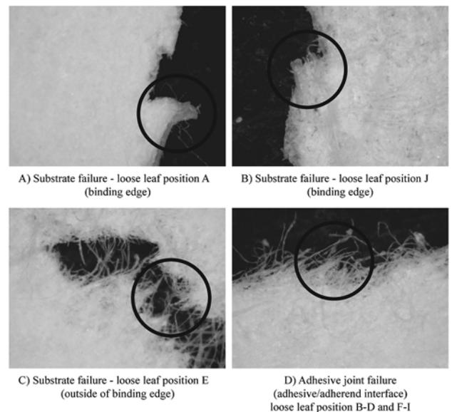
Figure 11 Paperback failure characterisation photographs. Photomicrographs under 200× magnification, showing loose leaf binding edge after testing
