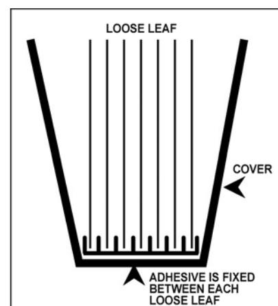
**Figure 1** Paperback - the binding edges filled with rigid adhesive
