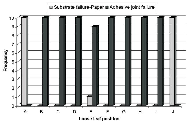
Figure 10 Visual assessment – Paperback failure characterization
