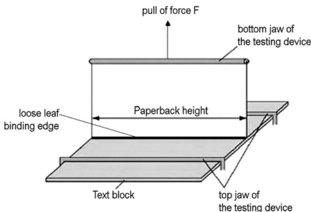
Figure 3 Adhesive joints strength measurement (pull test device)
