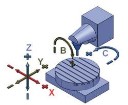
Figure 3 5D machine structure with tool rotation and workpiece rotation
