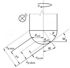
Figure 6 Longitudinal downward milling
