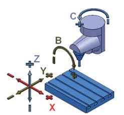
Figure 2 5D machine structure with tool rotation in two axes
