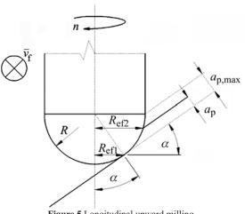
Figure 5 Longitudinal upward milling
