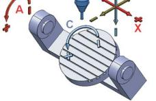
Figure 1 5D machine structure with swivel rotary table
