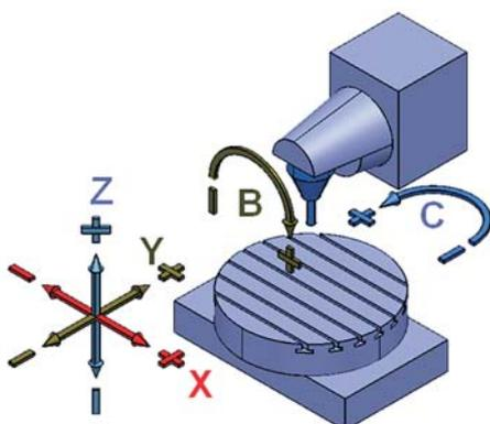
Figure 3 5D machine structure with tool rotation and workpiece rotation
