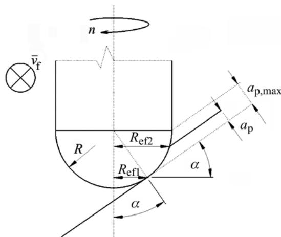
Figure 5 Longitudinal upward milling
