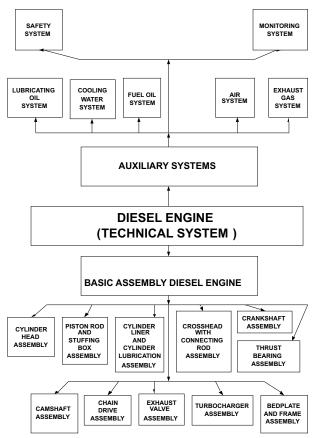
Figure 1 Schematic of ship propulsion system with relevant systems and sub-systems [3]
