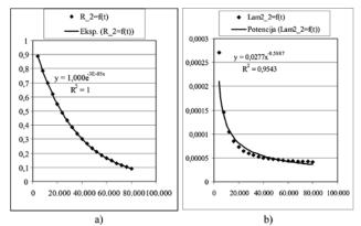
**Figure 11** Regression analysis for model II of ship propulsion system for status 2
