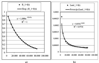
Figure 10 Regression analysis for model II of ship propulsion system for status 1
