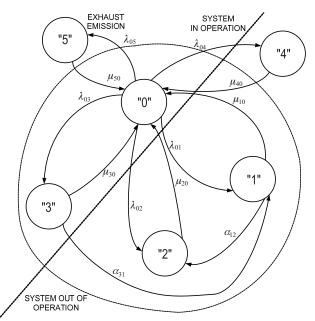
Figure 3 Markov model of ship propulsion system [3]
