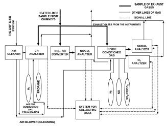
Figure 2 Schematic of data sampling for control and measurement of exhaust gas emission [3]
