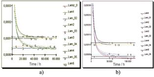
Figure 8 Diagram of malfunction intensity functions "Lam1, Lam2, Lam3, Lam4, Lam5" of ship propulsion system obtained by simulation and application of average times for
