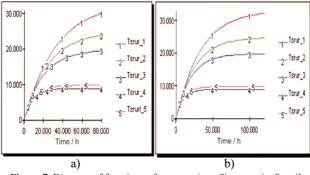
Figure 7 Diagram of functions of average times "in operation" until reaching one of the statuses "1, 2, 3, 4, 5" of ship propulsion system for a) scenario I (80 000 hours in operation)
