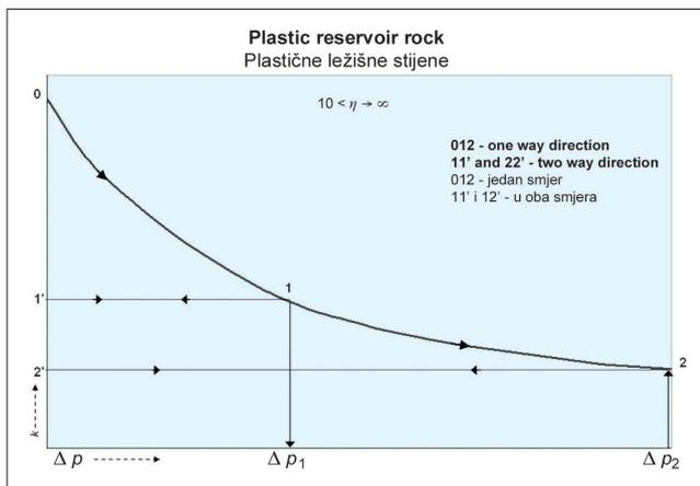
**Fig. 2b. Permeability against the pressure**
