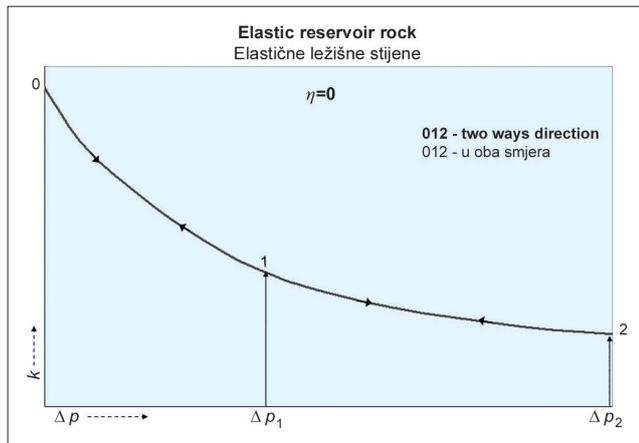
**Fig. 2a. Permeability against the pressure**
