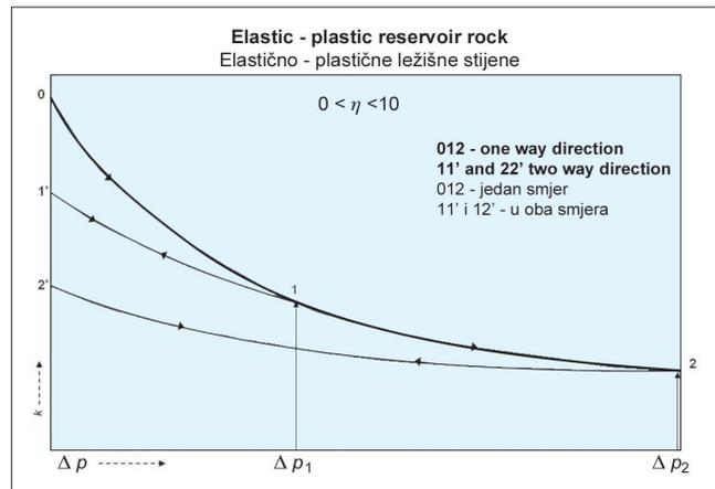
**Fig. 2c. Permeability against the pressure**
