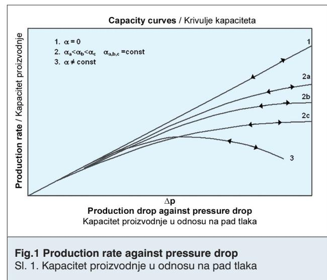
Fig.1 Production rate against pressure drop
