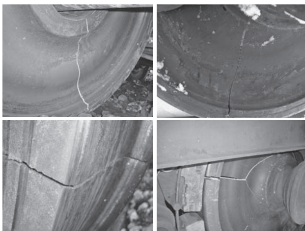
Figure 2 Typical examples of wheels braking [5]
