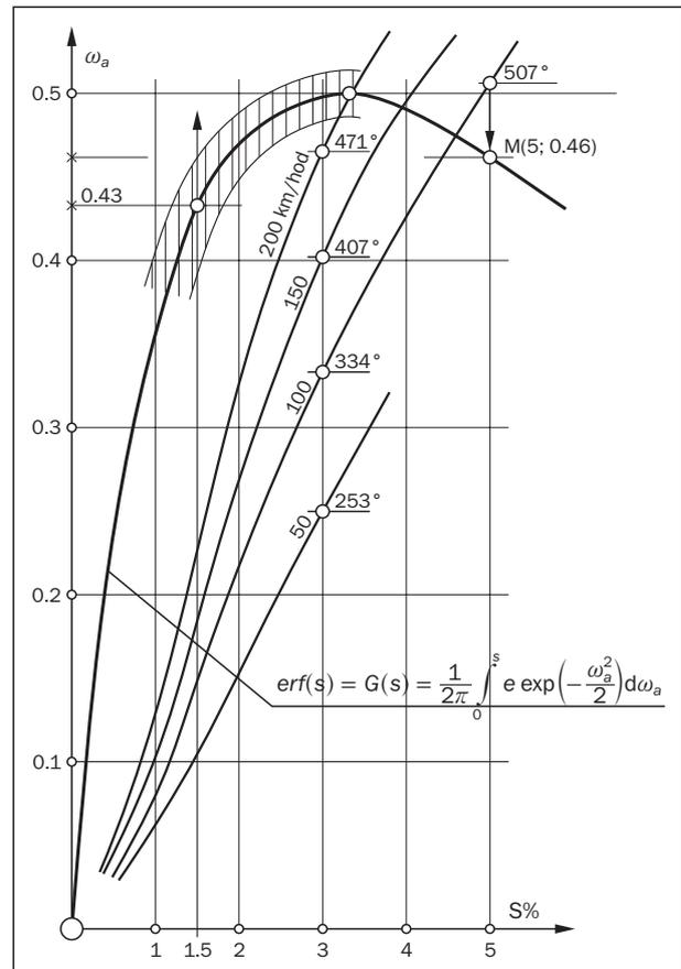
Figure 1 - Theoretical prediction of the contact temperatures  $T$ , drawn along the slip curve
