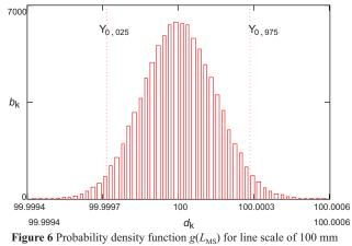
**igure 6** Probability density function  $g(L_{MS})$  for line scale of 100 mm where,  $\alpha_{MS}=10\times10^{-6}$  1/K
