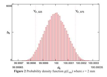
The estimated standard deviations of the output value  $L_{\rm MS}$  for line scale length of 100 mm amounts to 84 nm which confirms the uncertainty determined by the GUM method.
