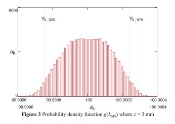
The estimated standard deviation of the output value  $L_{\rm MS}$  for line scale length of 100 mm where distance between points on laser head z = 3 mm amounts to 133 nm.
