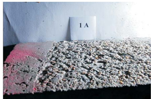
Figure 1 C 20/25 concrete, transition between uncurved concrete surface (left) and blasted concrete surface (right), pressure 130 MPa
