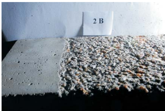
Figure 4 C 45/55 concrete, transition between uncured concrete surface (left) and blasted concrete surface (right), pressure 210 MPa
