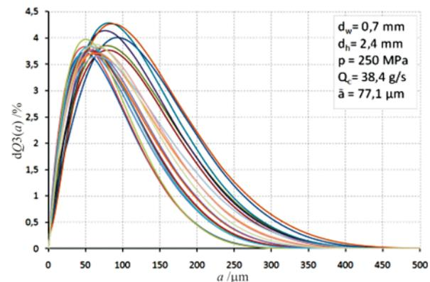
Figure 5 Distributions of hard coal particles fraction comminuted with water pressure of 250 MPa
