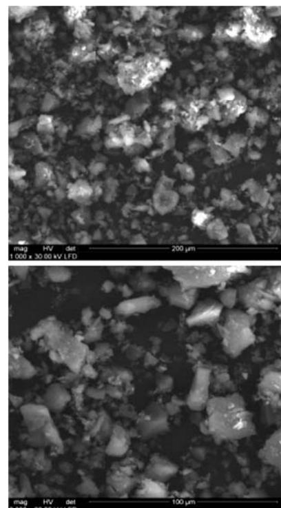
Figure 10 SEM images illustrating diversification of brown coal size and shape after high-pressure water jet comminution ( $p=250$  MPa)
