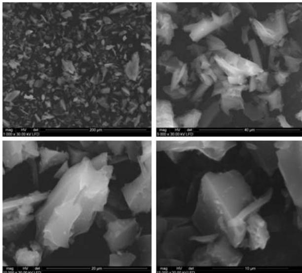
Figure 15 SEM pictures of charcoal showing different stages of their specific surface development
