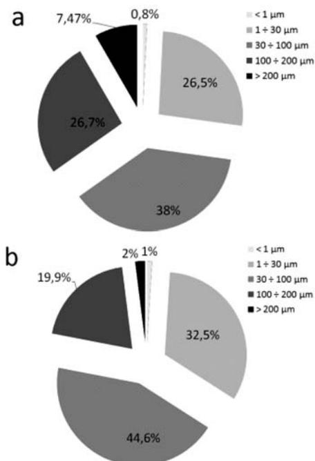
Figure 6 Quantitative contents of hard coal different fractions comminuted with high-pressure water jet (a - 150 MPa, b - 250 MPa)
