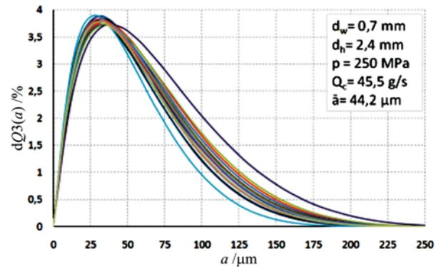
Figure 8 Distributions of brown coal particles fraction comminuted with water pressure of 250 MPa
