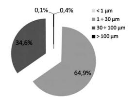
Figure 13 Quantitative contents of charcoal different fractions comminuted with high-pressure water jet (p= 250 MPa)
