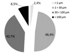
Figure 9 Quantitative contents of brown coal different fractions comminuted with high-pressure water jet (p= 250 MPa)
