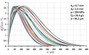
Figure 4 Distributions of hard coal particles fraction comminuted with water pressure of 150 MPa
