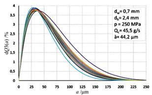
Figure 8 Distributions of brown coal particles fraction comminuted with water pressure of 250 MPa
