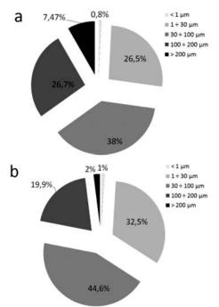
Figure 6 Quantitative contents of hard coal different fractions comminuted with high-pressure water jet (a - 150 MPa, b - 250 MPa)
