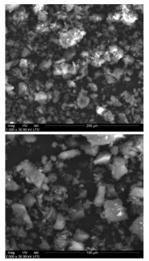
Figure 10 SEM images illustrating diversification of brown coal size and shape after high-pressure water jet comminution (p= 250 MPa)
