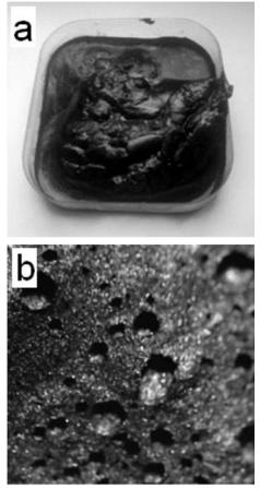
Figure 14 Air-dried charcoal mass (a) of great porosity (b), comminuted with high-pressure water jet (p=250 MPa)
