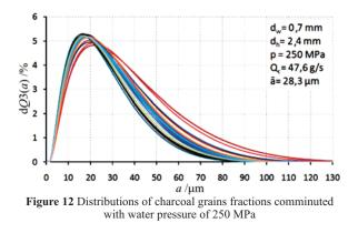
Hydrojetting comminution of fine charcoal gives highefficient micronization. Only the first stage of processing gives the range from approx. 65 % to over 83 % of charcoal comminuted with 250 MPa water jet to the range of  $1\div30$ µm. Detailed information on that results from the graph presented in Fig. 13.
