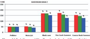
Figure 14 Red, Green and Blue Tone levels for the different finishing technologies of basalt surfaces
