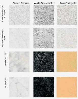
Figure 11 Appearance of some marble surfaces treated with different technologies
