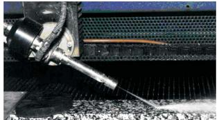
Figure 3 Picture of a typical test showing the features of the jet hitting the rock sample
