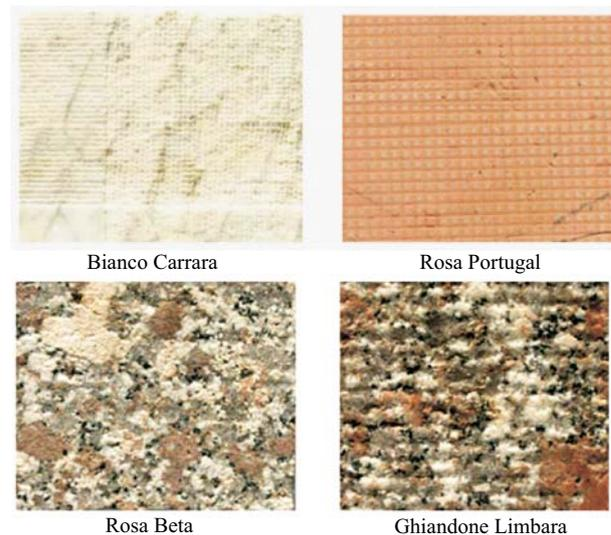
Figure 7 Influence of rock features on the results of waterjet treatment under different experimental conditions
