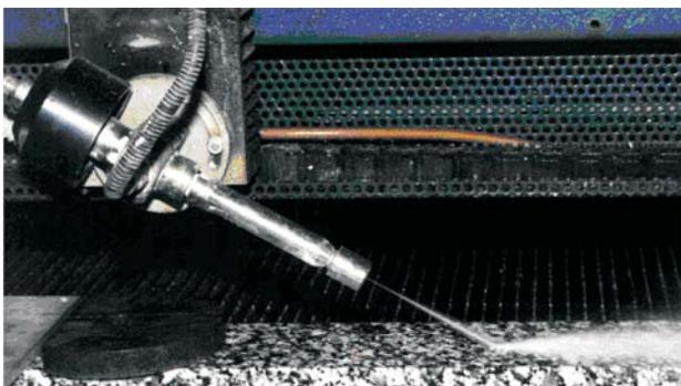
Figure 3 Picture of a typical test showing the features of the jet hitting the rock sample
