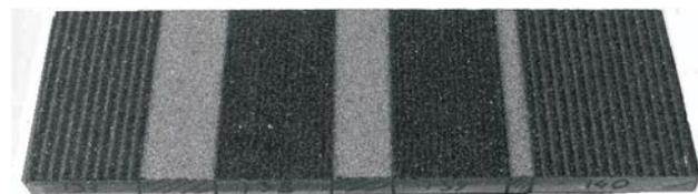
Figure 8 Different striation pattern on basalt (the pale grey parts correspond to the original blade sawing surface)
