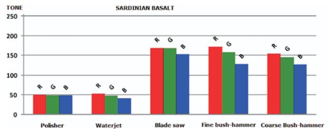
Figure 14 Red, Green and Blue Tone levels for the different finishing technologies of basalt surfaces
