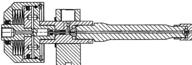
Figure 2 Details of the cutting head used for the experiments
