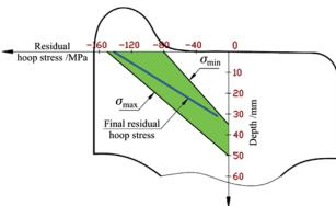
Firure 5 Final distribution of residual hoop stress below the tread of the railway wheel with respect to standard limits
