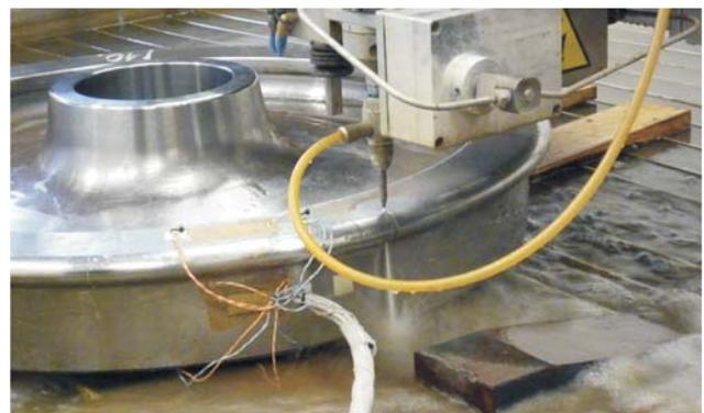
Figure 4 Cutting of railway wheel by abrasive water jet
