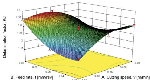
**Figure 12** The dependence of delamination factor on cutting parameters for HSS-Co twist drill
