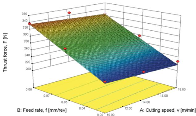
**Figure 6** The dependence of thrust force on cutting parameters for HSS-Co twist drill
