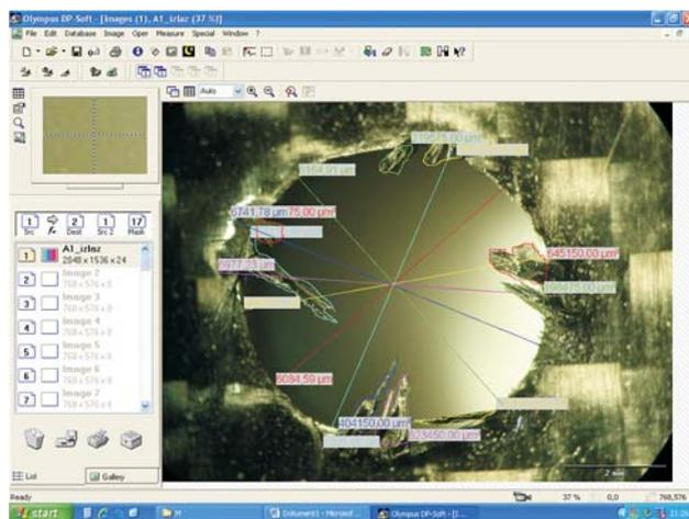
Figure 4 Screen of software used for measuring delamination
