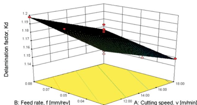
**Figure 13** The dependence of delamination factor on cutting parameters for MultiConstructional twist drill
