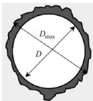
Figure 5 Scheme of delamination factor
