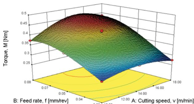
**Figure 11** The dependence of drilling torque on cutting parameters for "Brad & Spur" drill
