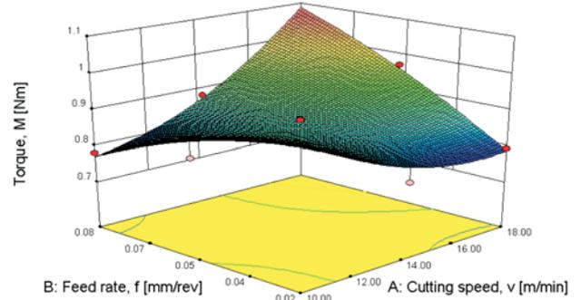
**Figure 9** The dependence of drilling torque on cutting parameters for HSS-Co twist drill
