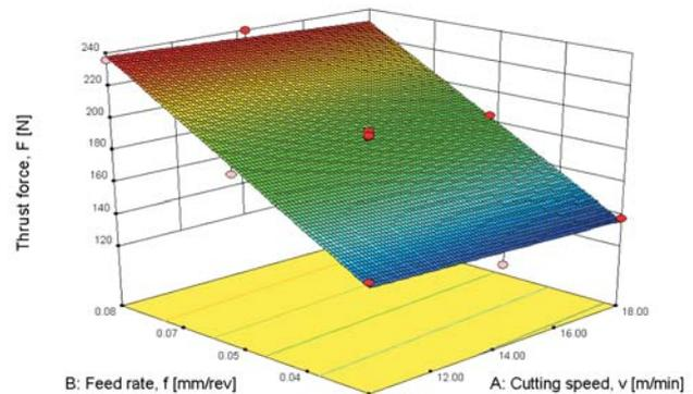
**Figure 7** The dependence of thrust force on cutting parameters for Multi Constructional twist drill
