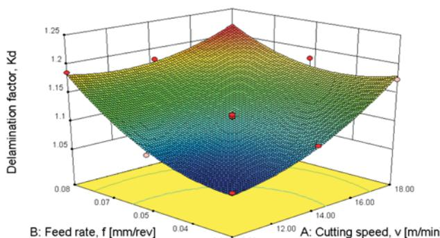
**Figure 14** The dependence of delamination factor on cutting parameters for "Brad & Spur" drill
