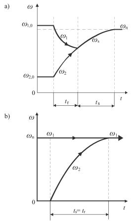
Figure 3 a) Process of the clutch engagement, with an internal combustion engine; b) Process of the clutch engagement, with an electric engine
