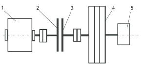
Figure 2 The test bench works with certain mass moved (1 - drive engine, 2 - driving parts of the clutch, 3 - working parts of the clutch, 4 - rotary mass and 5 - brake)
