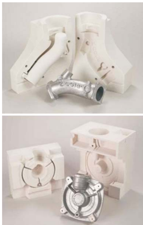
Figure 4 Examples of molds for direct casting of aluminum produced by 3D printing [13]
