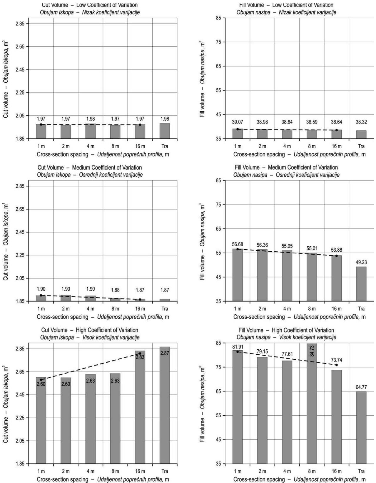
**Fig. 14** Cut and fill volumes estimated by the model for the road segments classified into three terrain ruggedness classes across different cross-section spacings
