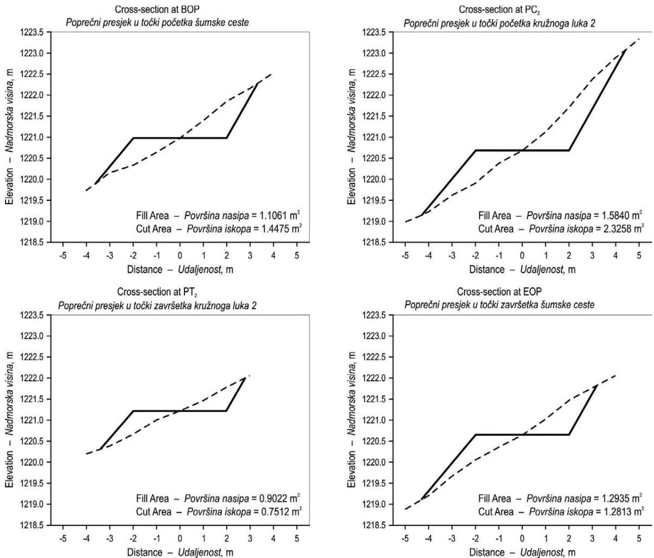
**Fig. 11** Cross-section diagrams obtained for the 3-SP hypothetical forest road
