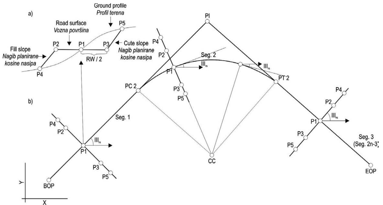
**Fig. 4** Cross-section design considered by the model (a), and road segment slopes ( $m_s$ ) used to identify the location of cross-section design points on straight and curved road segments (b)
