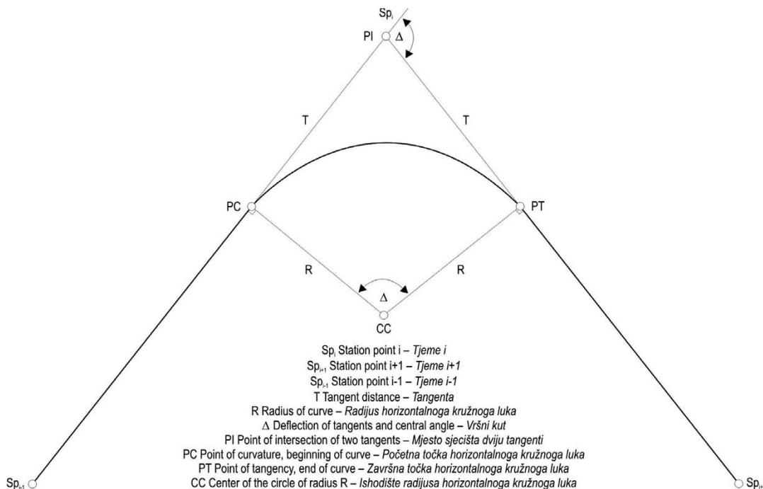
**Fig. 2** An example of horizontal curve design and nomenclature
