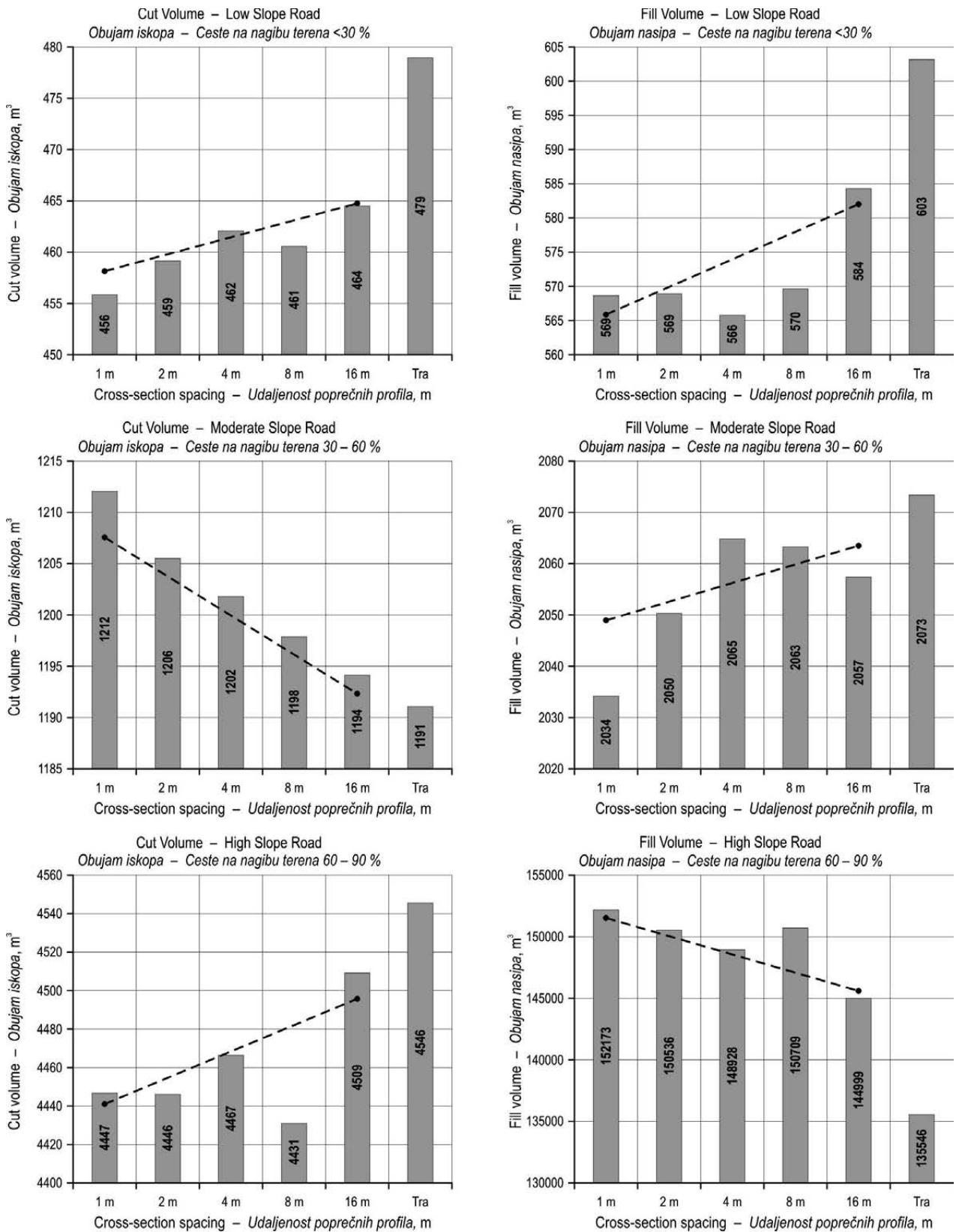
**Fig. 13** Cut and fill volumes estimated by the model for the three hypothetical 1 km forest roads at different cross-section spacings
