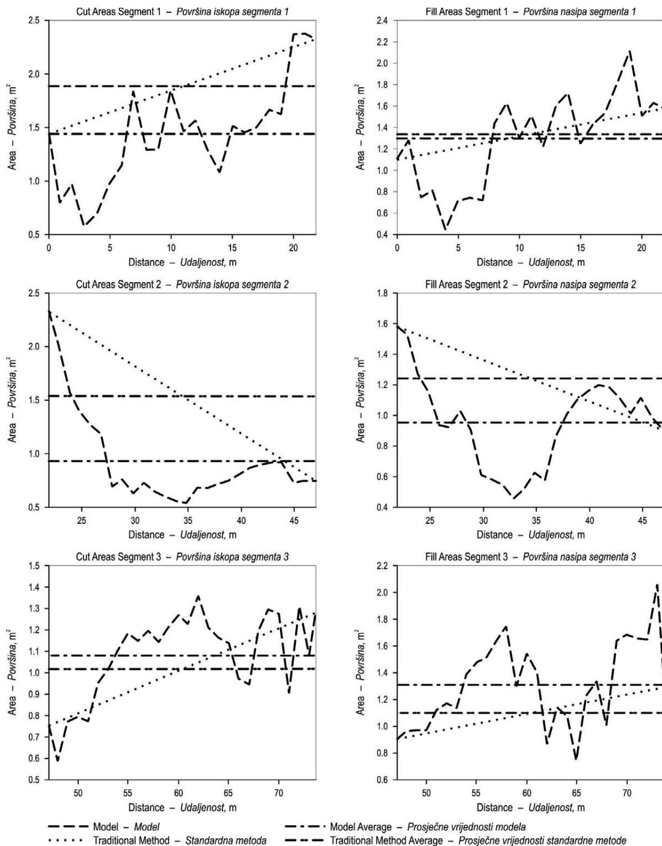
**Fig. 12** Cut and fill areas for the 3-SP hypothetical forest road calculated by the model and the traditional method
