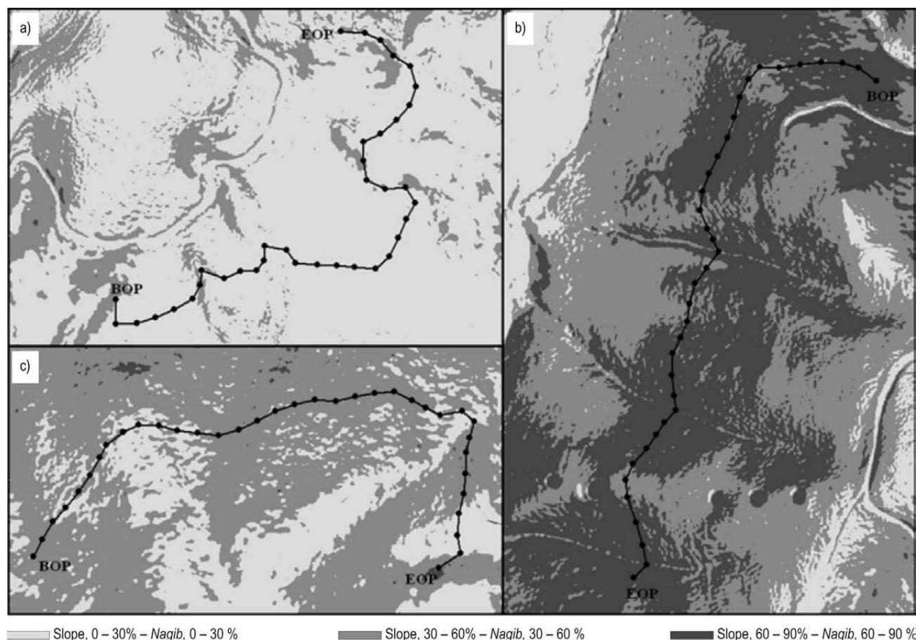
**Fig. 9** Layout of the three hypothetical 1 km forest roads located in low (a), moderate (b), and steep (c) slope areas
