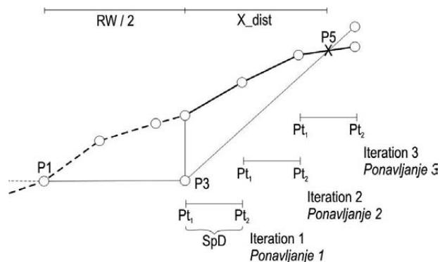
**Fig. 5** Iterative process performed by the model to identify the intersection point (P5) between the cut slope and ground surface
