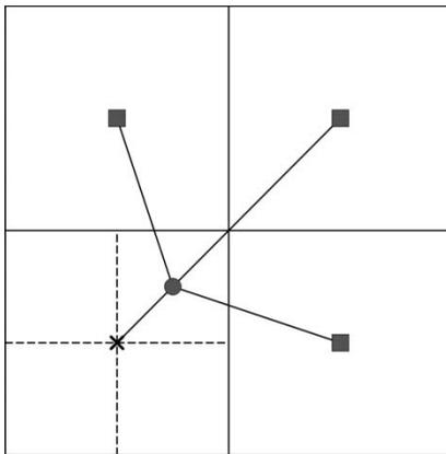
**Fig. 1** Estimating ground elevation on a given point (dot) using the interpolation method based on four grid cells including the grid cell containing the point (grid cell with a cross) and three adjacent grid cells (grid cells with squares)
