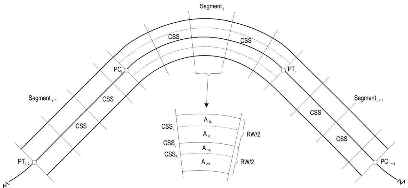
**Fig. 7** Cross sections taken from straight and curved road segments for earthwork volume estimation
