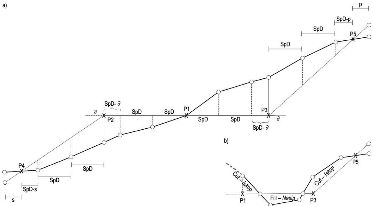
**Fig. 6** Cross-section design points used to calculate cut and fill areas (a), and an example of a cross-section having both fill and cut areas on one side of the road center line (P1) (b)
