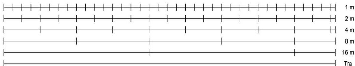
**Fig. 10** Number and location of cross-sections along a given straight road segment for different cross-section spacings (1, 2, 4, 8, and 16 meters)
