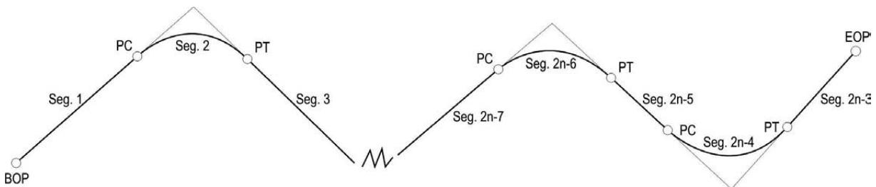
Fig. 3 Plan view of a proposed road including straight and curved road segments
