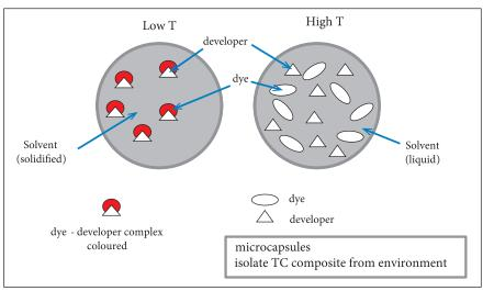
Figure 1. Schematic representation of leuco dye-developer solvent composite system
