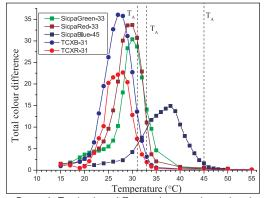
Figure 6. Total colour difference between heated and cooled states of the same TC sample as a function of temperature, as measured for TCXR-31, TCXB-31, SicpaRed-33, SicpaGreen-33 and SicpaBlue-45.
