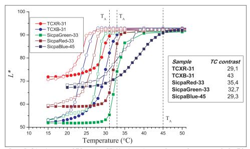
Figure 5. Colour hysteresis of TC samples. CIELAB colour values as a function of temperature for five TC samples: TCXR-31, TCXB-31, SicpaRed-33, SicpaGreen-33 and SicpaBlue-45 at heating (full signs) and cooling (open signs). Samples with similar layer thickness were evaluated. Efficiency of colour change is expressed by TC contrast, the total colour difference between totally coloured and discoloured states and is given in the key (in CIELAB units).
