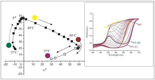
Figure 8. Changing of CIELAB values of irreversible TC ink printed on top of the blue thermochromic ink in (a\*,b\*) plane at heating, irreversible change, (solid signs) and cooling, reversible change, (open signs). Small figure represents reflectance spectra of irreversible TC inks printed on top of the blue TC ink.
