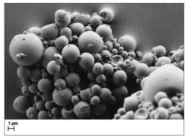
Figure 2. SEM micrograph of a microencapsulated thermochromic composite
