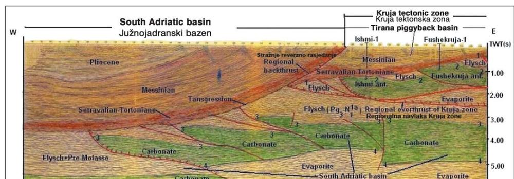
Fig. 9. Migrated seismic line 6-6 (according to geological cross-section in Ishmi area at Fig. 6)
