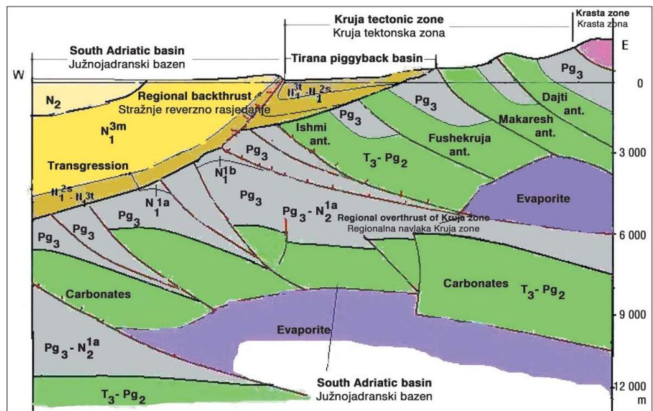
**Fig. 7. Schematic geological cross-section in Ishmi area**
