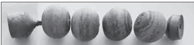
Figure 11 Balls obtained in the process of cross rolling with upsetting conducted at the Lublin University of Technology
