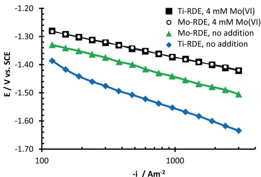
**Figure 3.** IR-corrected polarization curves recorded in 1 M NaOH, 70°C at a rotation rate of 5000 rpm. All polarization curves were recorded in the anodic direction. The electrodes were pre-polarized at  $-3 \text{ kA m}^{-2}$  for 15 min prior to the polarization curves.
