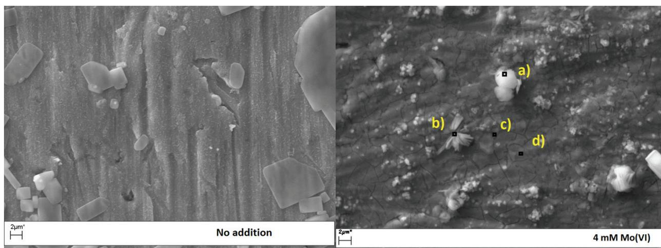
**Figure 4.** SEM images on Ti-RDEs polarized for 30 min at  $-3 \text{ kA m}^{-2}$  in 2 M NaCl,  $\text{pH} \approx 6.5$  and 70°C with and without 4 mM Mo(VI). The rotation rate during polarization was 3000 rpm. The composition was analyzed with EDS in atomic % and the relative Mo/(Mo+Ti) atomic ratio was in the marked points: a.) 23 %, b) 26 %, c.) 6 %, d.) 9 %
