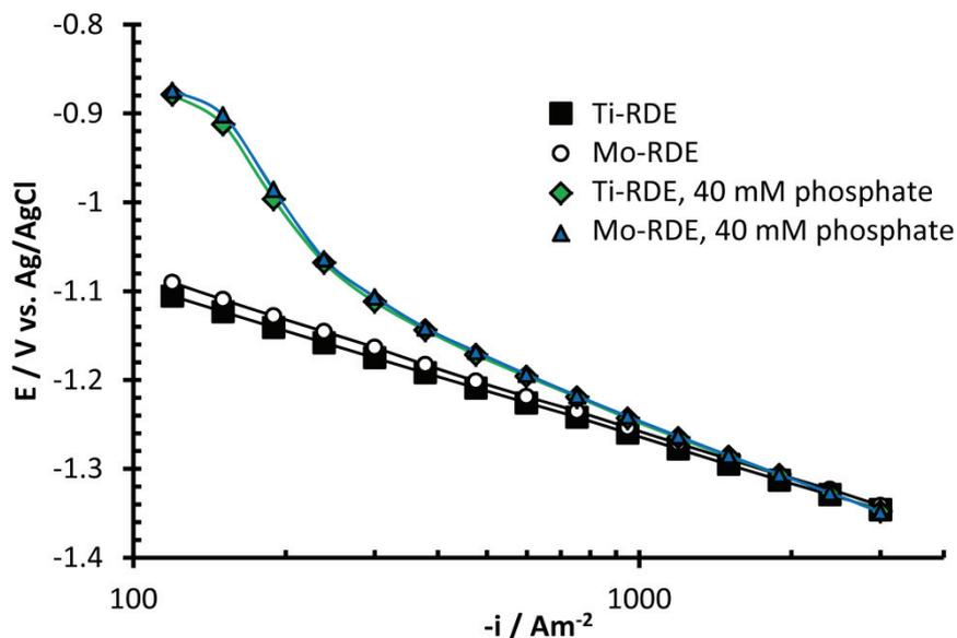
**Figure 2.** IR-corrected polarization curves recorded in 2 M NaCl, 4 mM Mo(VI), pH=6.5, 70°C at a rotation rate of 5000 rpm. All polarization curves were recorded in the anodic direction. The electrodes were pre-polarized at  $-3 \text{ kA m}^{-2}$  for 15 min prior to the polarization curves.
