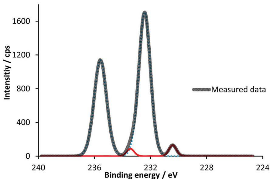
**Figure 8.** XPS spectrum of the Mo 3d signal with resolved peaks in the outermost surface layer of a Ti-RDE polarized for 30 min in 1 M NaOH, 4 mM Mo(VI), 70°C at  $-3 \text{ kA m}^{-2}$  and a rotation rate of 3000 rpm.
