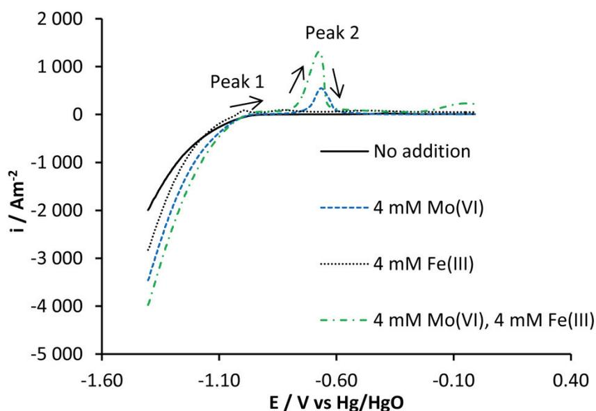
**Figure 9.** Potential sweeps recorded on a platinum RDE in 1 M NaOH, 70°C at a sweep rate of  $50 \text{ mV s}^{-1}$  and a rotation rate of 5000 rpm. The electrode was pre-polarized at  $-3 \text{ kA m}^{-2}$  for 30 min prior to the polarization curves. Concentrations given for Fe(III) correspond to the added amount since some precipitation was observed.
