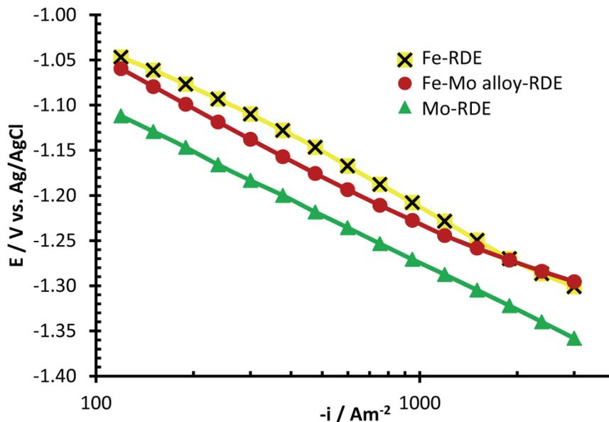
**Figure 13.** IR-corrected polarization curves recorded in 2 M NaCl, pH 6.5, 70°C at a rotation rate of 5000 rpm. All polarization curves were recorded in the anodic direction. The electrodes were pre-polarized at  $-3 \text{ kA m}^{-2}$  for 1 min prior to the polarization curves.
