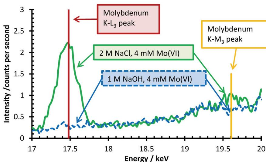
**Figure 6.** XRF-spectra for Ti-RDEs polarized for 30 min at  $-3 \text{ kA m}^{-2}$ ,  $70^\circ\text{C}$  and a rotation rate of 3000 rpm. The pH was adjusted to 6.5 for the electrolyte containing 2 M NaCl, 4 mM Mo(VI).
