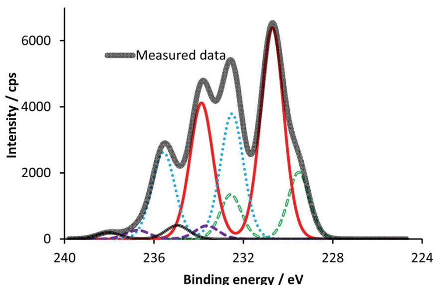
**Figure 7.** XPS spectrum of the Mo 3d signal with resolved peaks observed in the outermost surface layer of a Ti-RDE polarized for 30 min in 2 M NaCl, 4 mM Mo(VI), pH $\approx$ 7, 70°C at  $-3 \text{ kA m}^{-2}$  and a rotation rate of 3000 rpm.
