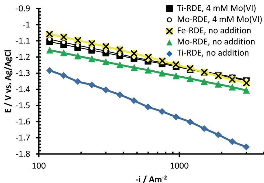
**Figure 1.** IR-corrected polarization curves recorded in 2 M NaCl, pH≈6.5, 70°C at a rotation rate of 5000 rpm. All polarization curves were recorded in the anodic direction. The electrodes were pre-polarized at  $-3 \text{ kA m}^{-2}$  for 15 min prior to the polarization curves.
