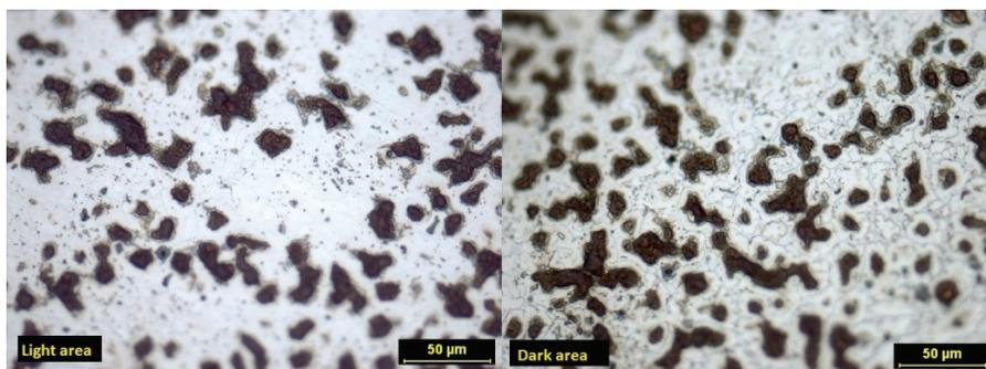
Figure 11. Optical microscopy images of the cast iron-molybdenum alloy. To the left is an image of a lighter area and to the right an image of a darker area on the surface, see Figure 10.
