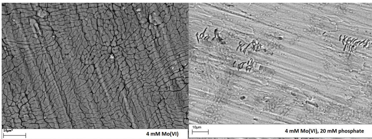
**Figure 5.** SEM images on Ti-RDEs polarized for 30 min at  $-3 \text{ kA m}^{-2}$  in 2 M NaCl, 4 mM Mo(VI),  $\text{pH}\approx 6.5$  and  $70^\circ\text{C}$  with and without 20 mM phosphate. The rotation rate during polarization was 3000 rpm.
