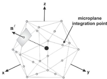
Figure 1. Discretization of a unit sphere
