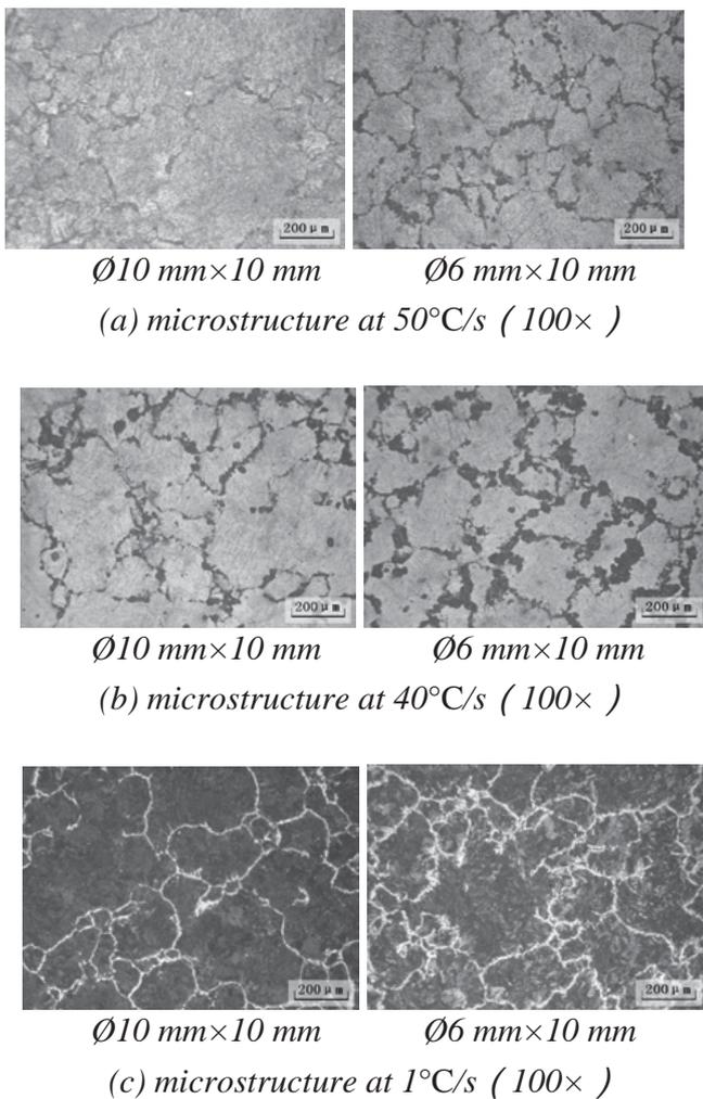
Figure 6. Microstructures at the specimen core
