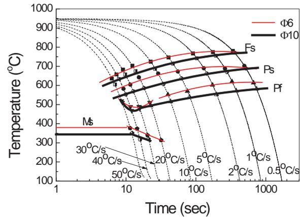
Figure 1. CCT curves of the  $\text{Ø}6 \text{ mm}$  and  $\text{Ø}10 \text{ mm}$  specimens, where Fs - ferrite start; Ps - pearlite start; Pf - pearlite finish; Ms - martensite start
