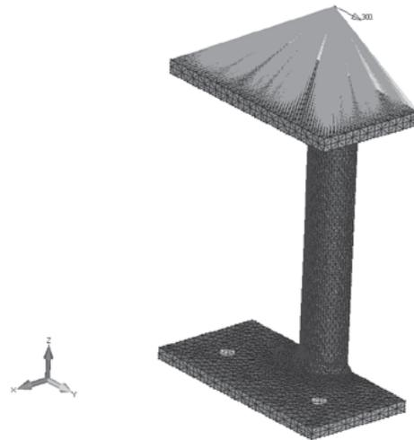
Figure 8. FE mesh of T-joint with rigid element
