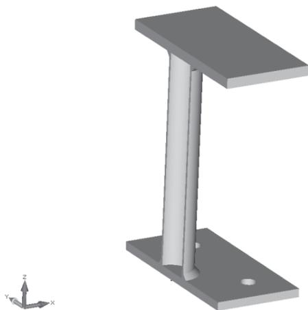
Figure 7. Half model of CHS-plate T-joint
