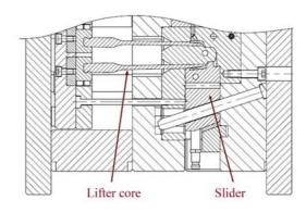
FIGURE 9 – Sliders and lifter cores
