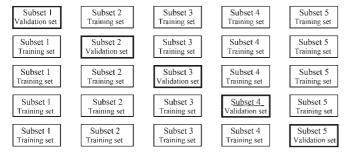
FIGURE 11 – Multifold cross-validation on 5 subsets
