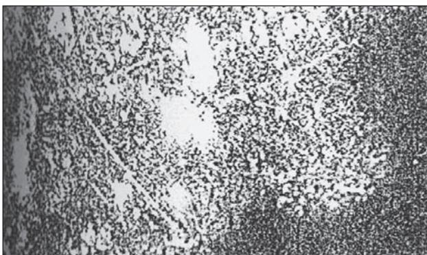
**Figure 13** Pearlitic structure with an uneven distribution of ferrite and cementite
