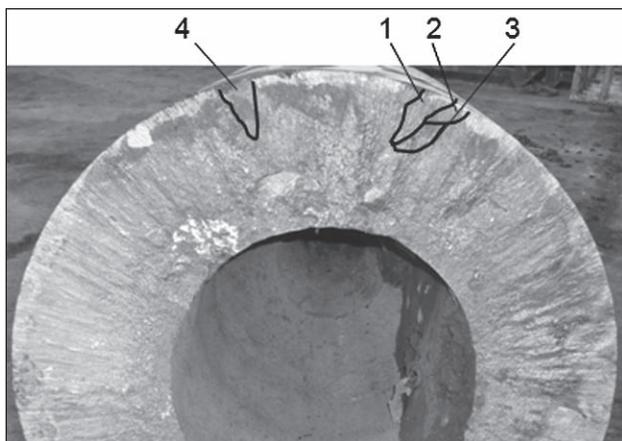
Figure 1 Worn tool and sampling areas
