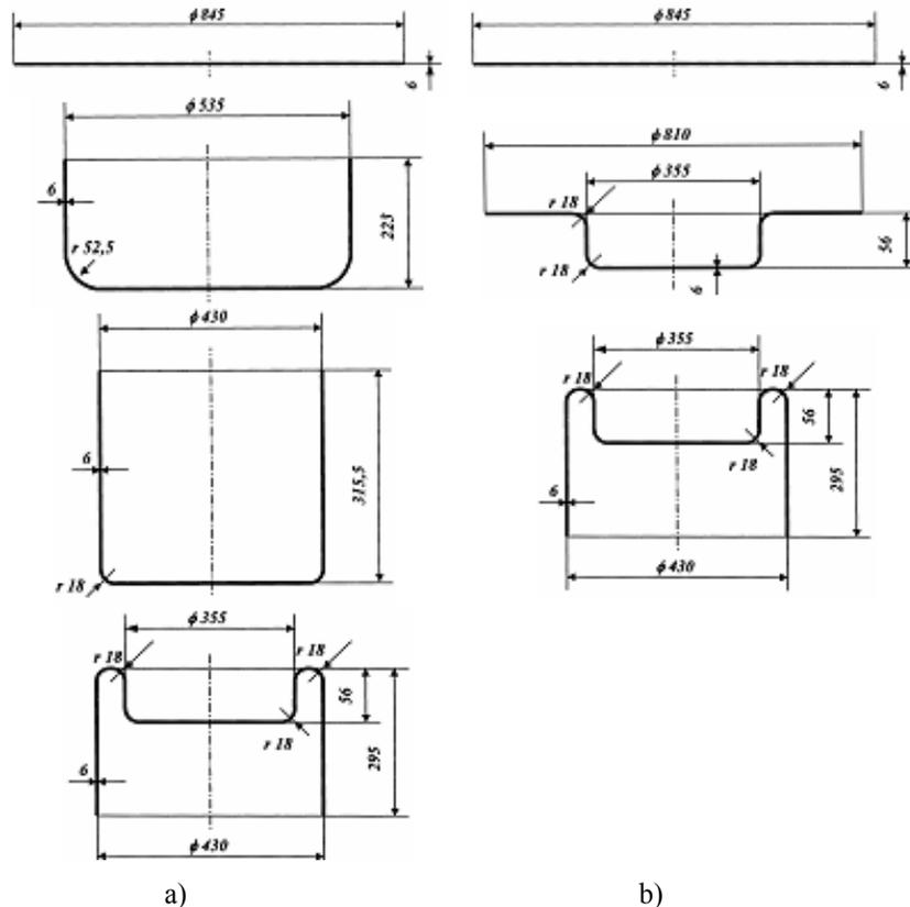
**Figure 10.** Variants of deep-drawing of the same cylindrical cup with a double wall: a) in three operations, b) in two operations
