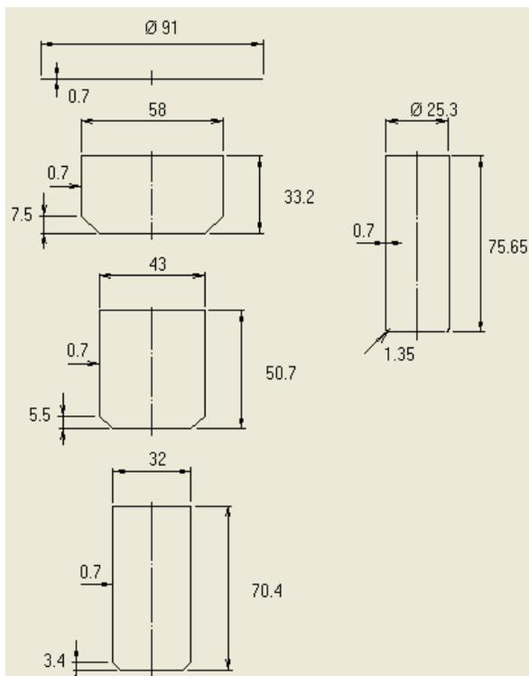
**Figure 6.** Deep-drawing process displayed in the DDCP
