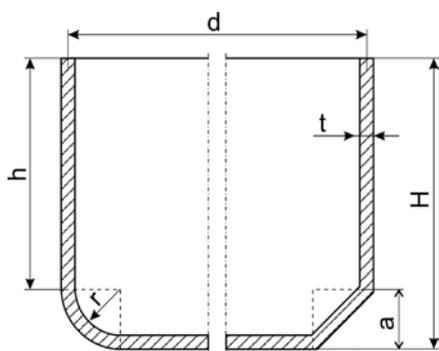
Figure 1. Cylindrical cup without flange: Variant I (left), Variant II (right)
