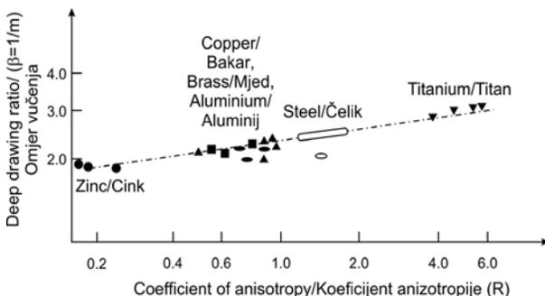
**Figure 8.** Influence of normal anisotropy on DDR
