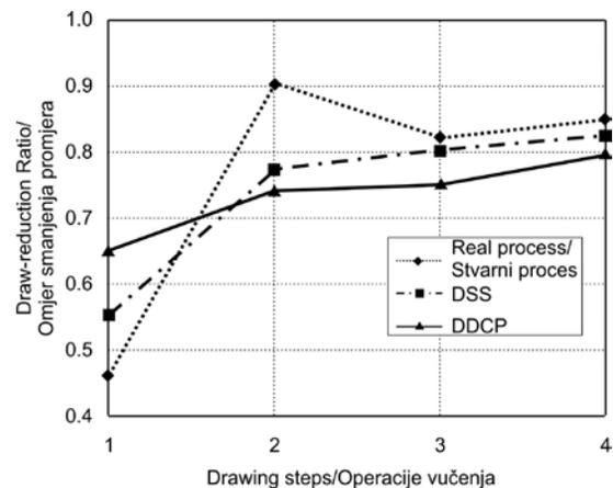
**Figure 7.** Graphical comparison between the DRR of the real process and output from the DDCP and DSS:  $D_0 = 91.9$  mm (real process),  $D_0 = 91.0$  mm (DDCP),  $D_0 = 92.4$  mm (DSS)
