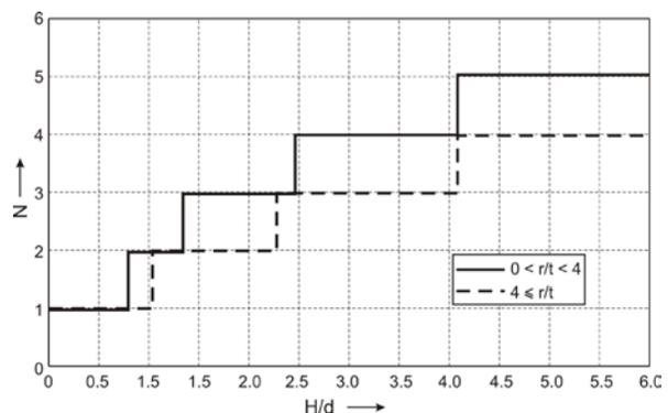
Figure 4. Number of deep-drawing steps vs. relative cup height
