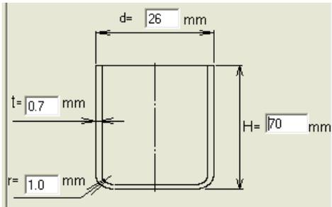
**Figure 5.** Cylindrical cup after deep-drawing process
