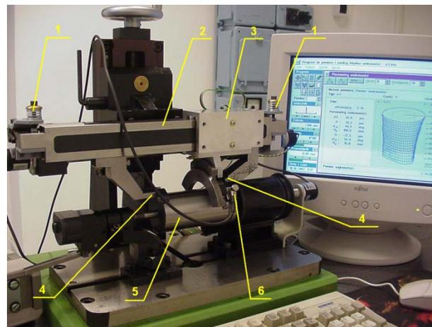
**Figure 3.** Model measuring device PSA 6 for the V-block method cylindricity measurements
