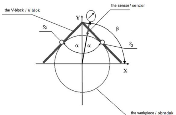
Figure 1. Concept of the V-block roundness measurement
