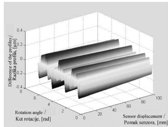
**Figure 9.** The difference of the model profile and the profile with the considered computational error caused by the V-blocks angles difference
