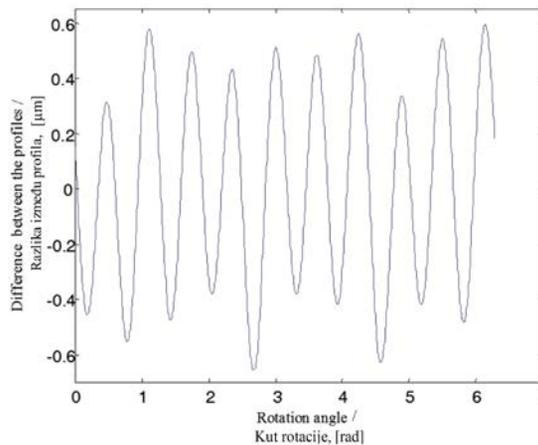
**Figure 6.** The difference between the profiles  $R_{\beta_n}(\varphi, z)$  and  $R_{\beta_r}(\varphi, z)$  in one of the cross-sections of the analyzed cylinder
