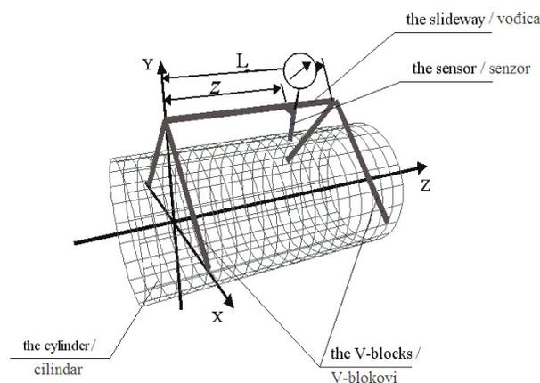
**Figure 2.** Concept of the V-block cylindricity measurement [28]
