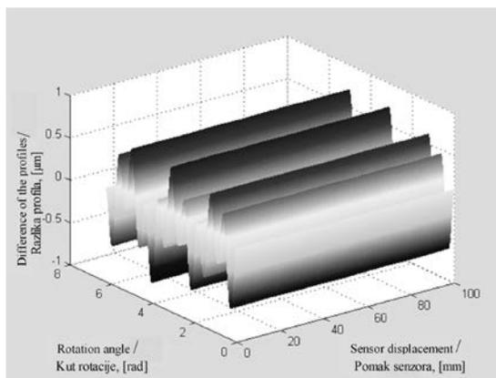
**Figure 8.** The difference between the model profile and the profile obtained through the simulation of the error of  $\alpha$
