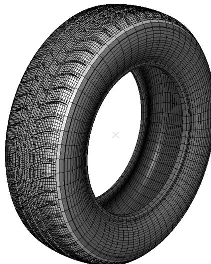
**Figure 5.** Final 3D FE model of the tire
