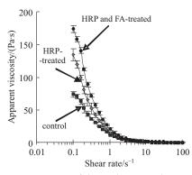
**Fig. 3.** Apparent viscosity of the yoghurt samples prepared from the skimmed milk (control) and skimmed milk treated with HRP only, or with HRP and FA and stored at 4 °C for 36 h as a function of shear rate
