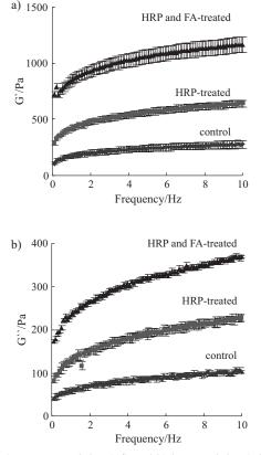
**Fig. 5.** a) storage modulus (*G*') and b) loss modulus (*G*") of the yoghurt samples prepared from the skimmed milk (control) and skimmed milk treated with HRP only, or with HRP and FA and stored at 4 °C for 36 h
