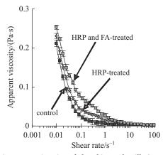
Fig. 1. Apparent viscosity of the skimmed milk (control) and skimmed milk treated with HRP only, or with HRP and FA as a function of shear rate
